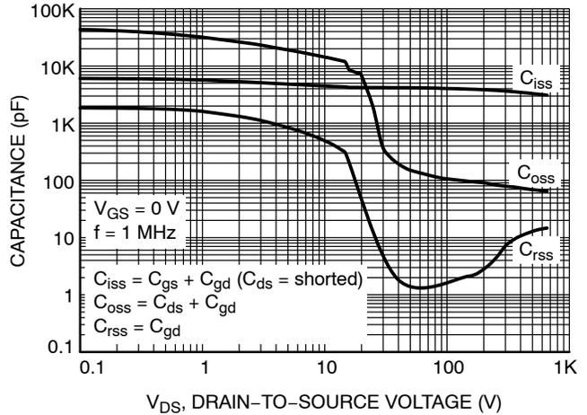
Figure 6. Capacitance Characteristics
