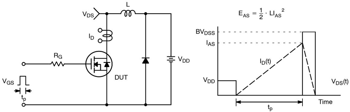
Figure 21. Unclamped Inductive Switching Test Circuit & Waveforms
