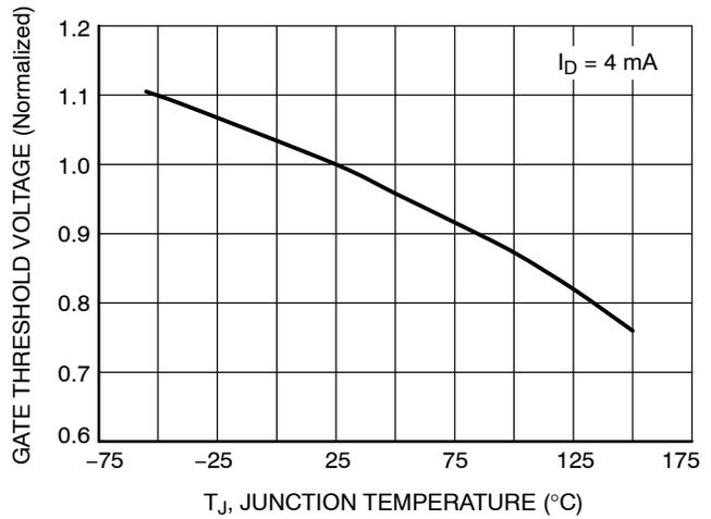
Figure 16. Normalized Gate Threshold Voltage vs. Temperature
