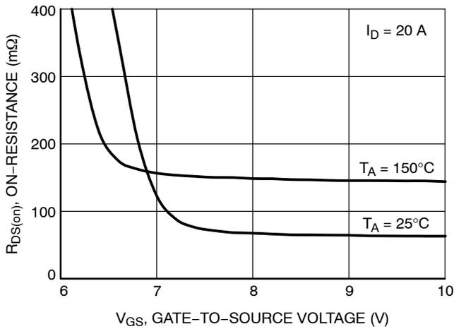
Figure 15. R<sub>DS(on)</sub> vs. Gate Voltage
