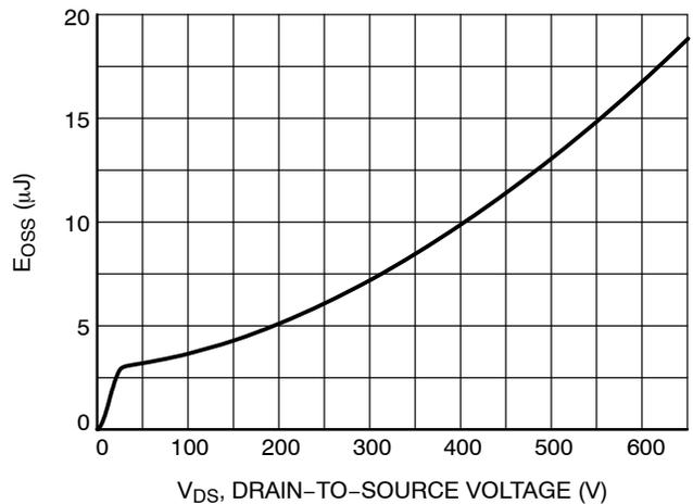
Figure 12. E<sub>OSS</sub> vs. Drain-to-Source Voltage
