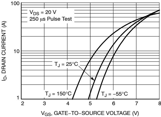
Figure 3. Transfer Characteristics
