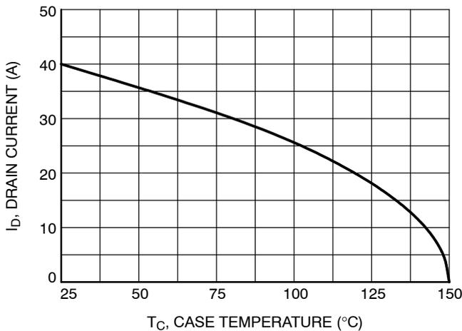
Figure 11. Maximum Drain Current vs. Case Temperature
