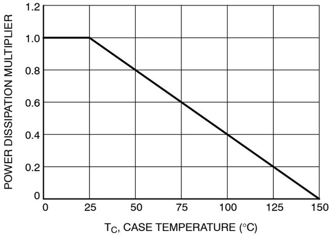
Figure 13. Normalized Power Dissipation vs. Case Temperature
