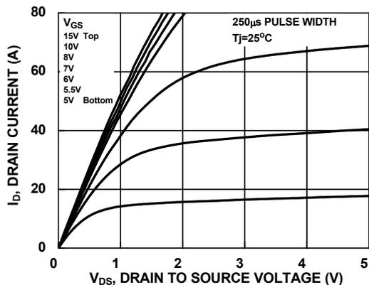
Figure 9. Saturation Characteristics
