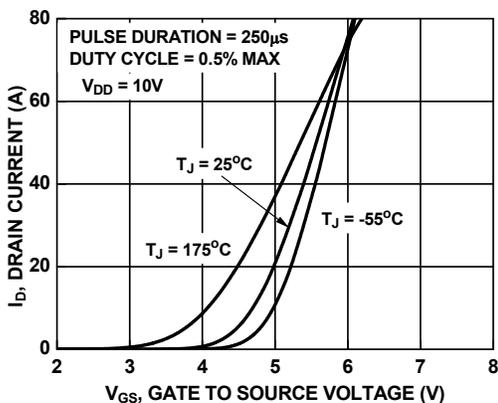
Figure 7. Transfer Characteristics
