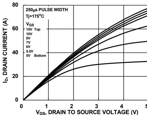
Figure 10. Saturation Characteristics
