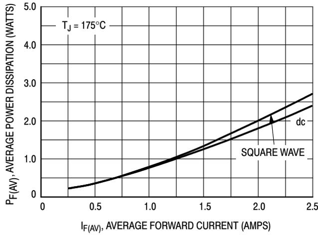
Figure 7. Power Dissipation
