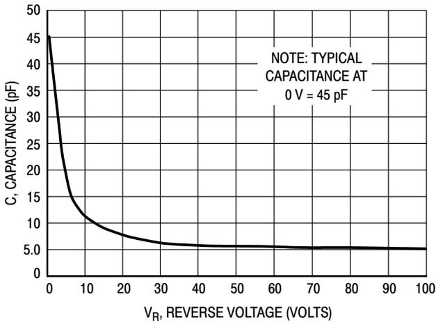
Figure 5. Typical Capacitance
