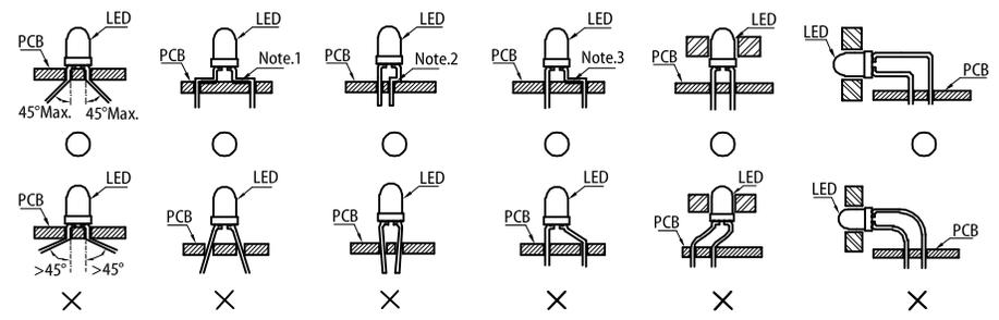
Note 1-3: Do not route PCB trace in the contact area between the leadframe and the PCB to prevent short-circuits.
