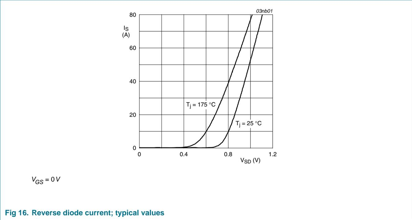
Fig 16. Reverse diode current; typical values
