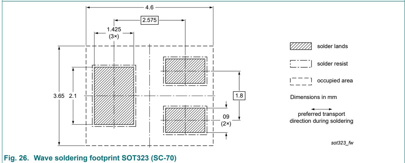
Fig. 26. Wave soldering footprint SOT323 (SC-70)
