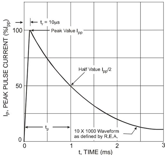
Figure 3 Pulse Waveform
