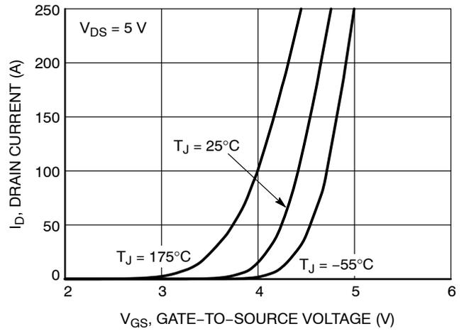
Figure 2. Transfer Characteristics
