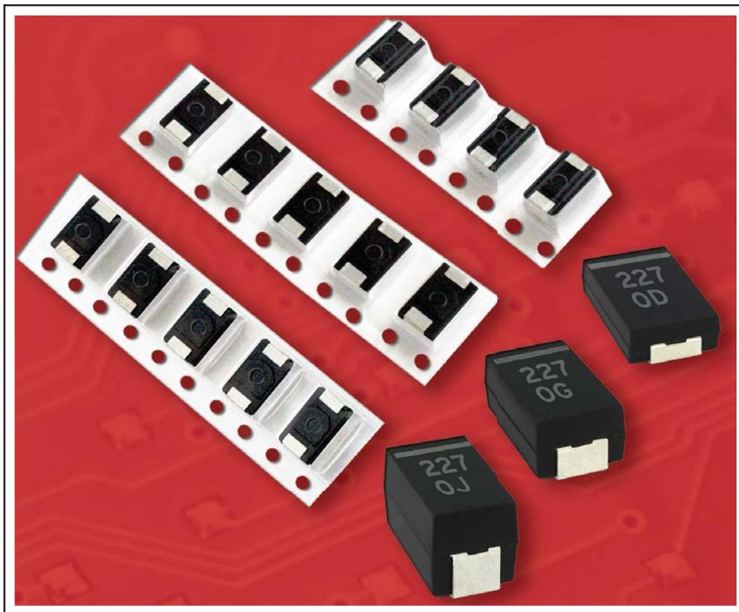
Murata Manufacturing Co., Ltd.'s ECAS series of polymer aluminum electrolytic capacitors realize low ESR, low impedance and high capacitance by means of multilayered aluminum foil for anode, solid conductive polymer for cathode.
