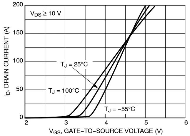
Figure 2. Transfer Characteristics
