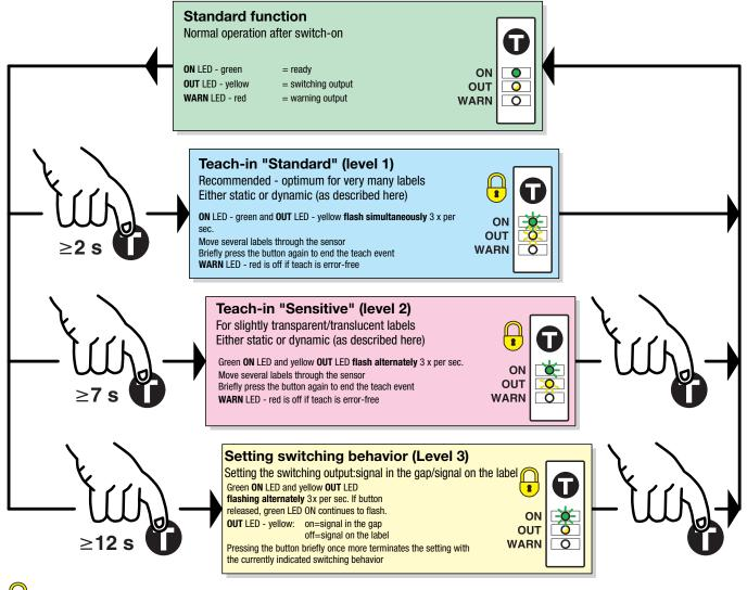
= function lockable through constant application of U<sub>B</sub> on the teach input (for devices with teach input only)
