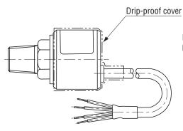
Please make sure that the drip-proof cover is properly placed over the main body and the cable.
