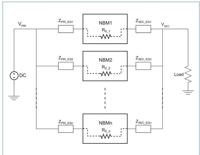
Figure 25 — NBM parallel array
