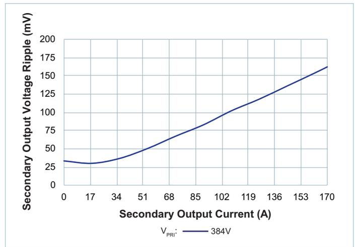
Figure 13 —  $V_{SEC\_OUT\_PP}$  vs.  $I_{SEC\_DC}$ ; No external  $C_{SEC\_OUT\_EXT}$ .
