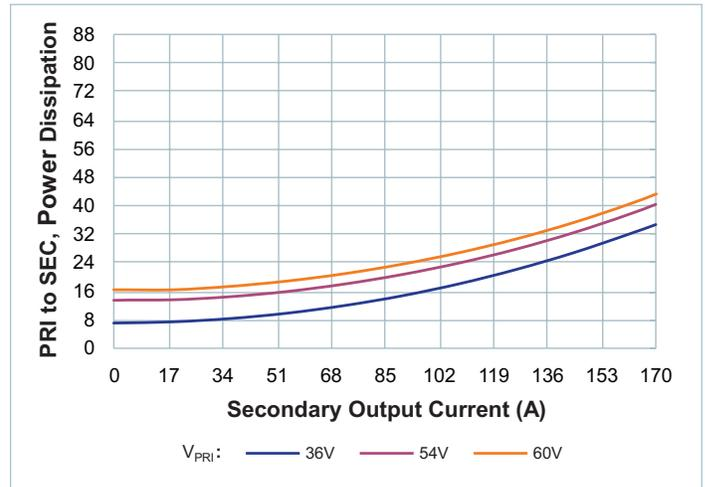
Figure 7 — Power dissipation at  $T_{CASE} = -40^{\circ}C$
