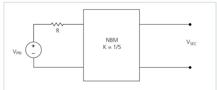
Figure 20 — K = 1/5 NBM with series primary resistor
