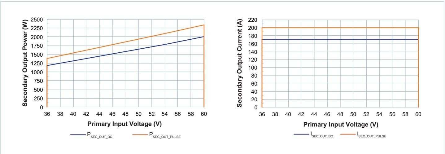
Figure 2 — Specified electrical operating area using rated  $R_{SEC\_HOT}$
