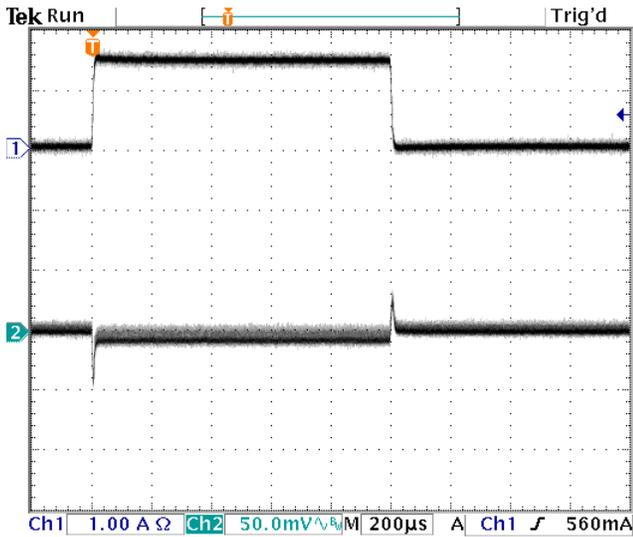
**Transient Response:  $V_{IN} = 5.0V$ ,  $V_{OUT} = 1.2V$ ,
