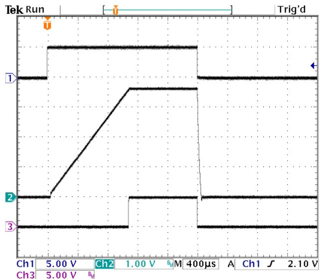
**Startup and Shutdown Waveform
