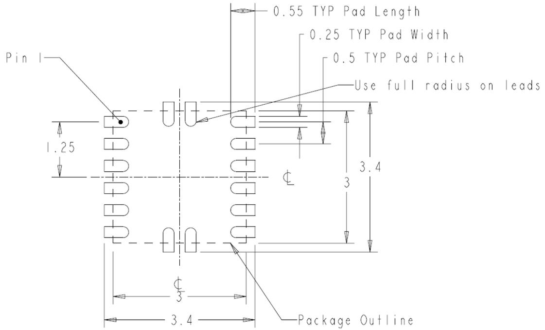
**Figure 8. EP53F8QI PCB Footprint (Top View)**
