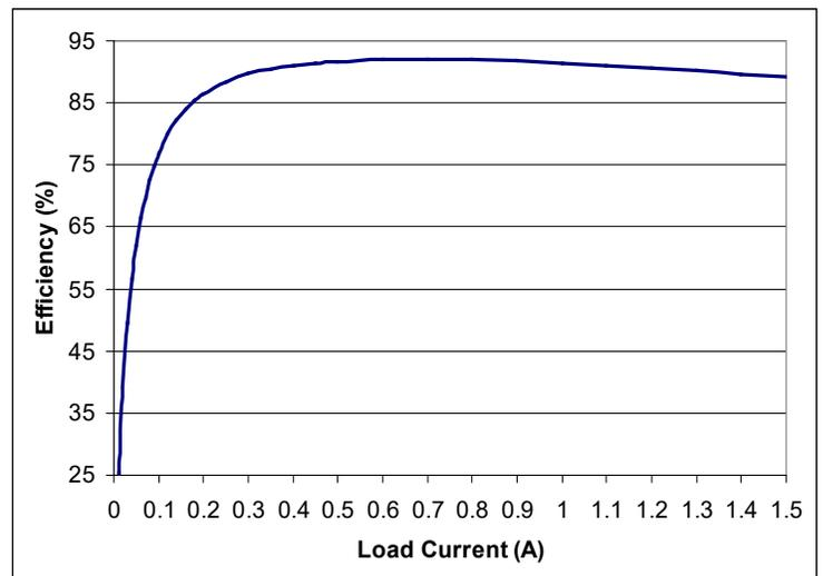
Figure 2. Efficiency, V<sub>IN</sub>=5V, V<sub>OUT</sub>=3.7V
