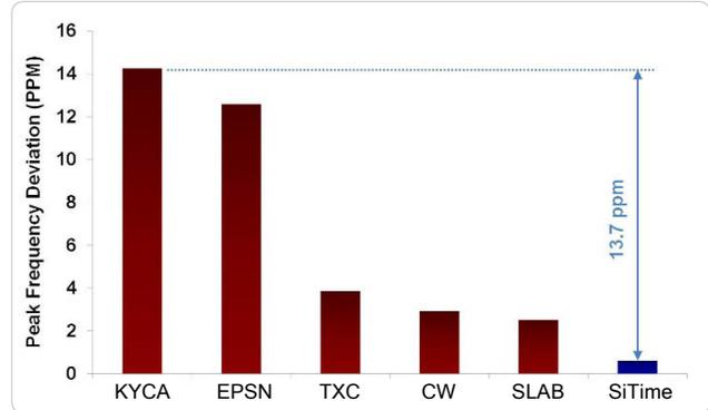
Figure 6. Shock Robustness<sup>[6]</sup>
