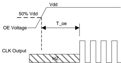
T\_oe: Time to re-enable the clock output
