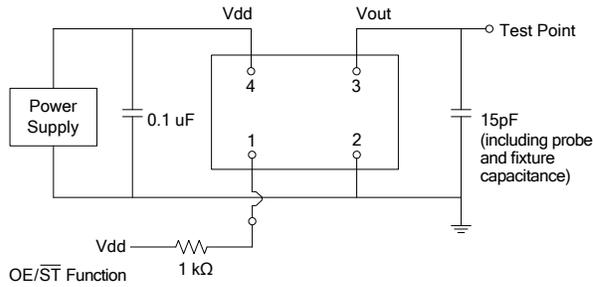
**Figure 2. Test Circuit**
