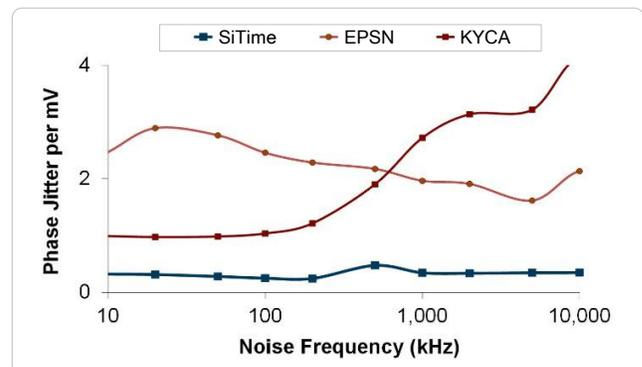
Figure 4. Power Supply Noise Rejection<sup>[4]</sup>
