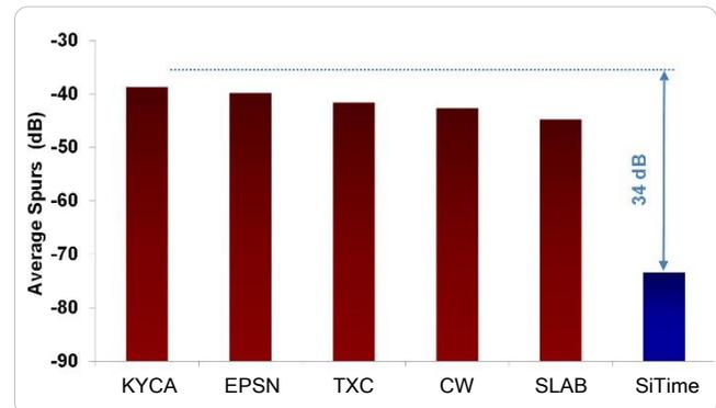
Figure 3. Electro Magnetic Susceptibility (EMS)<sup>[3]</sup>
