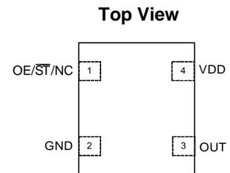
**Figure 1. Pin Assignments**
