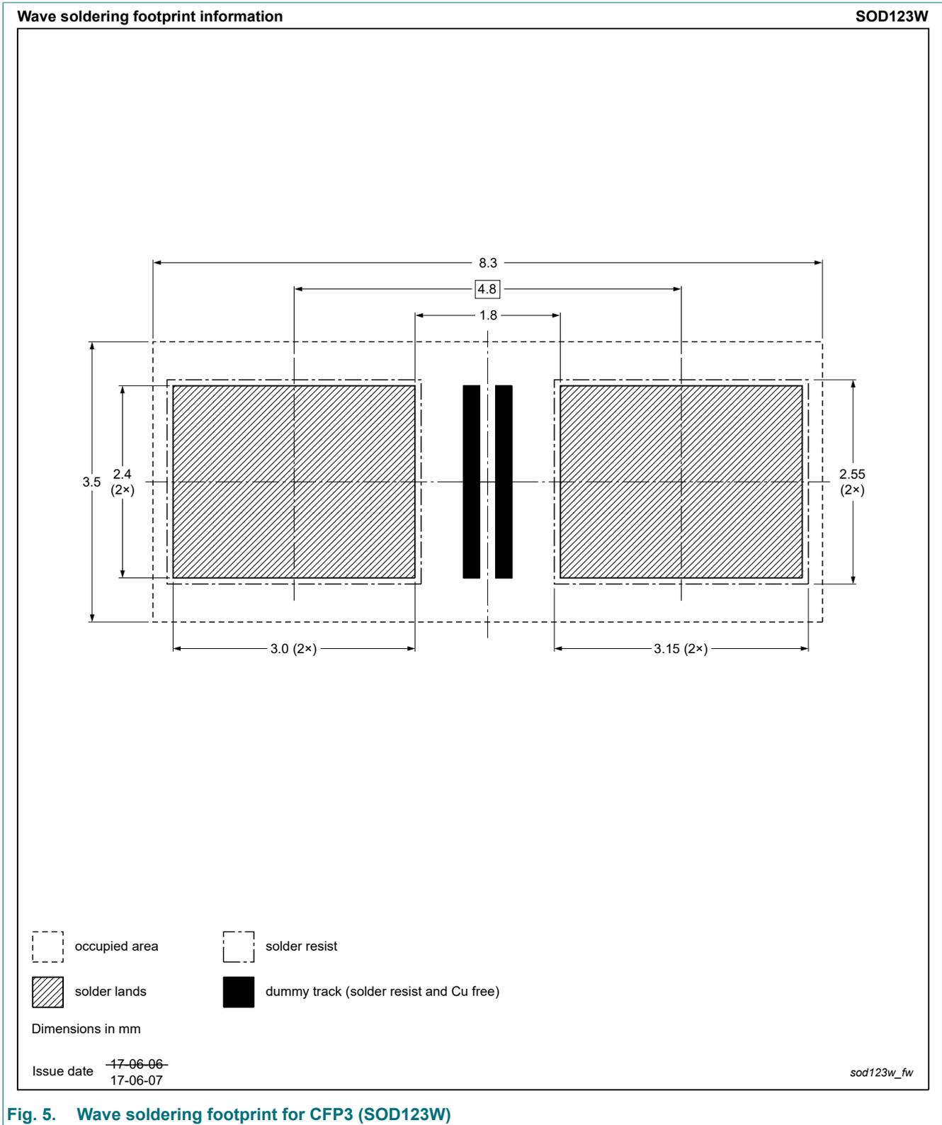
**Fig. 5. Wave soldering footprint for CFP3 (SOD123W)**
