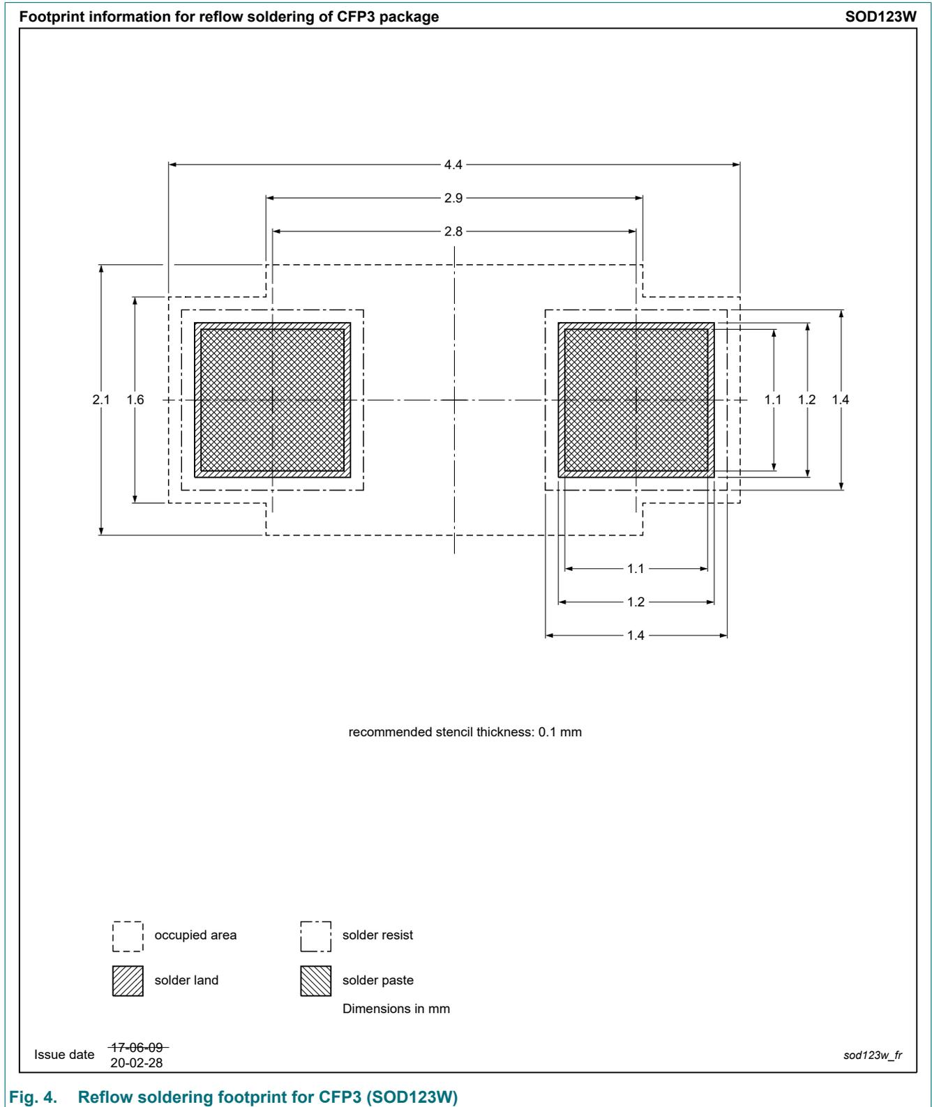
Fig. 4. Reflow soldering footprint for CFP3 (SOD123W)
