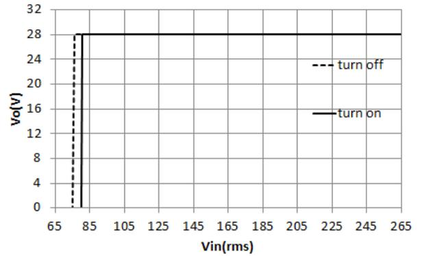
**Figure 2:**  $V_{out}$  vs.  $V_{in}$  @ Full load
