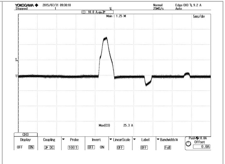
**Figure 8:** Inrush current @ Vin=220Vac
