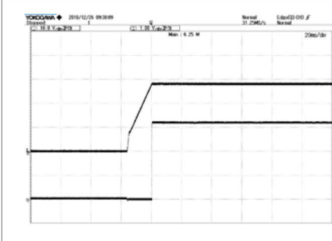
**Figure 9:** PG voltage vs. Vout @ Vin=220Vac, 0A Iout
