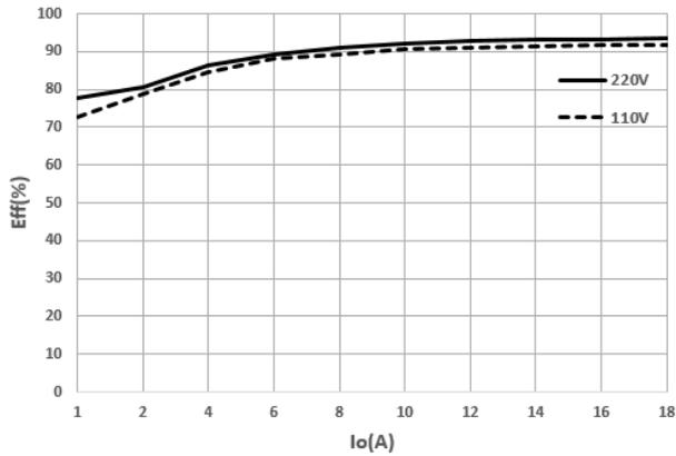
**Figure 1:** Efficiency vs. Output current @  $V_{in}=110,220VAC$
