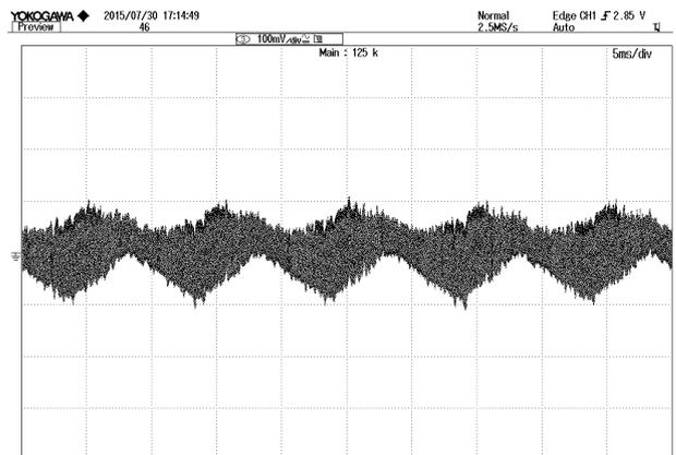
**Figure 6:** Output ripple & noise at  $110/220Vac$ ,  $18A I_{out}$
