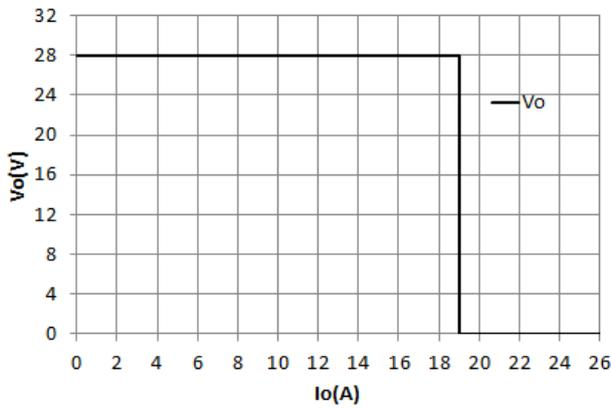
**Figure 3:** Output voltage vs. Output current @  $V_{in}=110,220VAC$
