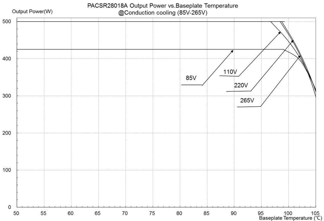
**Figure 14:** Thermal derating curve
