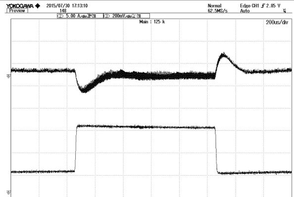
**Figure 4:** Dynamic response to load step 25%~75% with  $0.1A/uS$  slew rate at  $110/220Vac$
