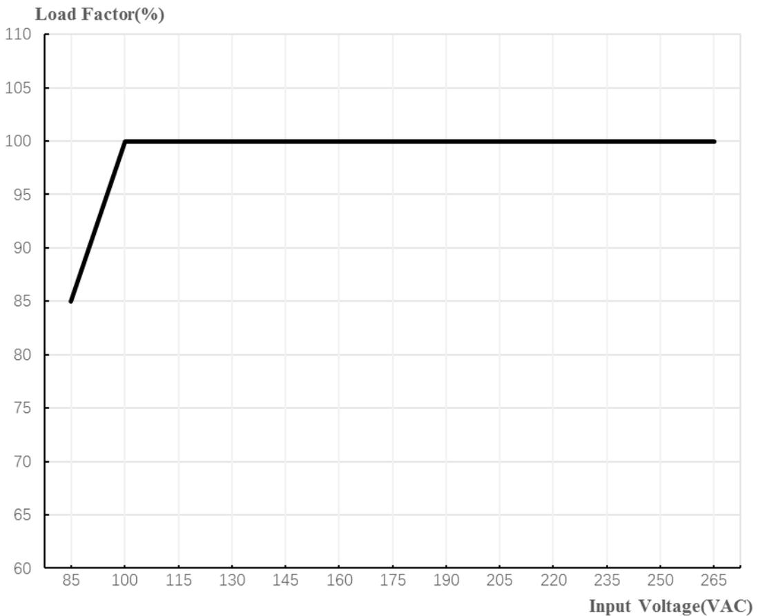
Figure 11: Input voltage derating curve
