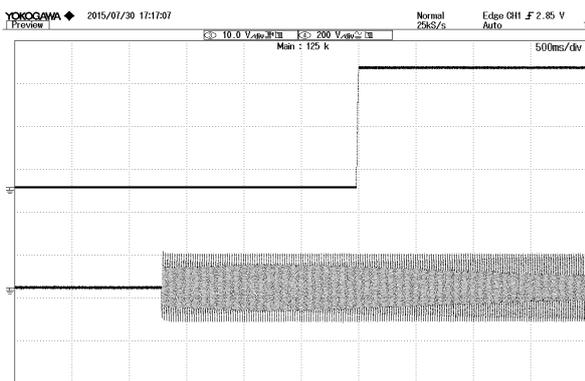
**Figure 5:**  $V_{out}$  start up with Enable on at  $110Vac$ ,  $18A I_{out}$ ,
