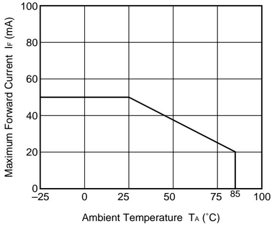
MAXIMUM LOAD CURRENT vs. AMBIENT TEMPERATURE
