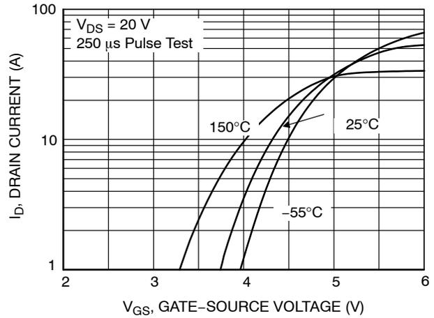
Figure 2. Transfer Characteristics
