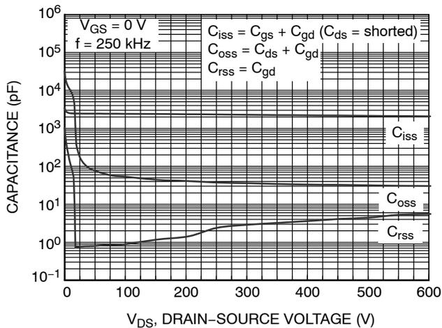
Figure 5. Capacitance Characteristics
