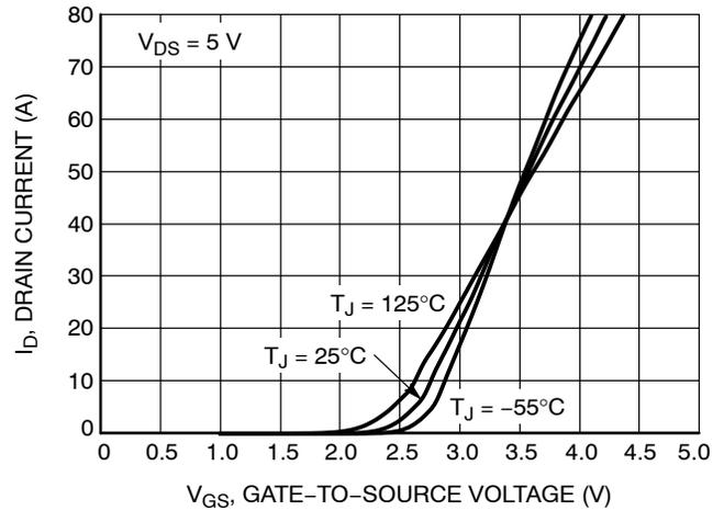
Figure 2. Transfer Characteristics
