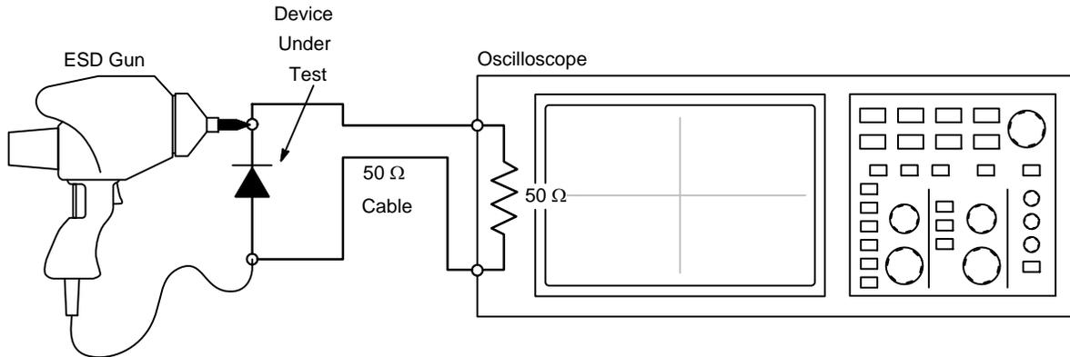
Figure 9. Diagram of ESD Clamping Voltage Test Setup
