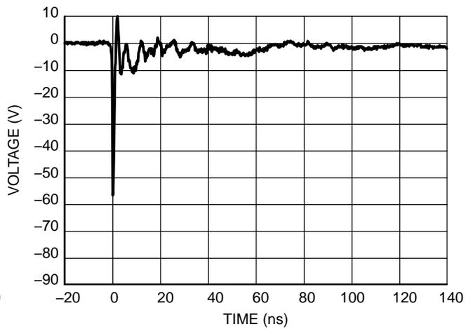
Figure 7. IEC61000-2-4 -8 kV Contact Clamping Voltage
