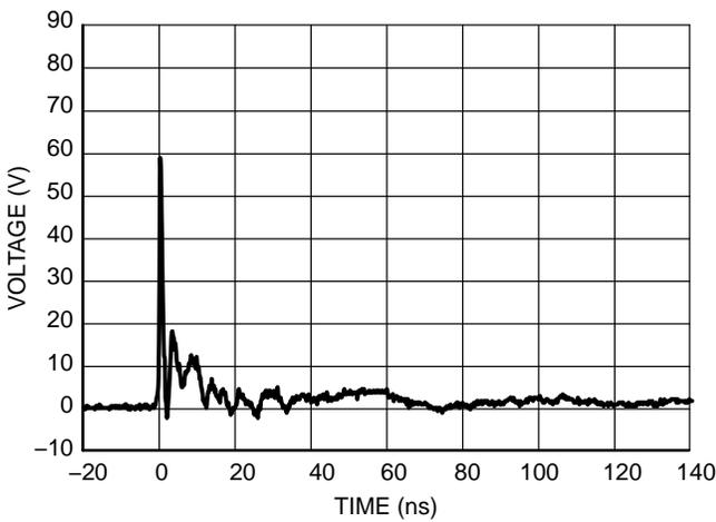
Figure 6. IEC61000-2-4 +8 kV Contact Clamping Voltage
