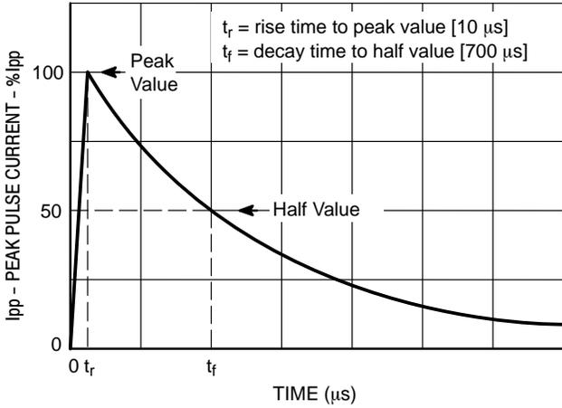
Figure 4. IEC61000-4-5 10/700  $\mu$ s Pulse Waveform
