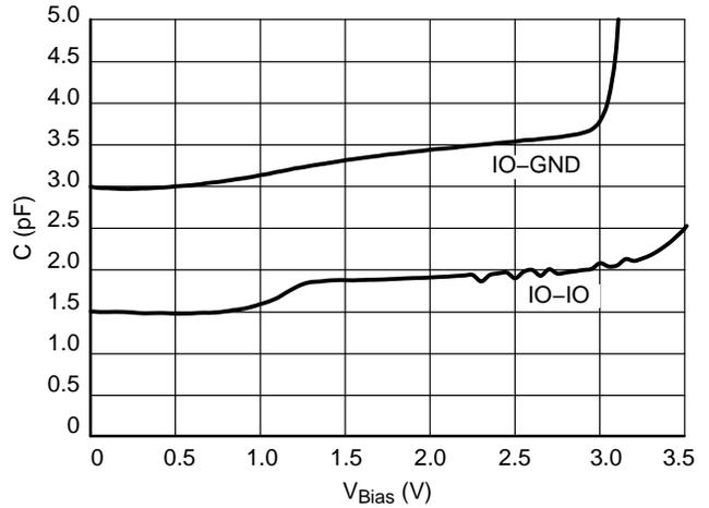
Figure 15. CV Characteristics
