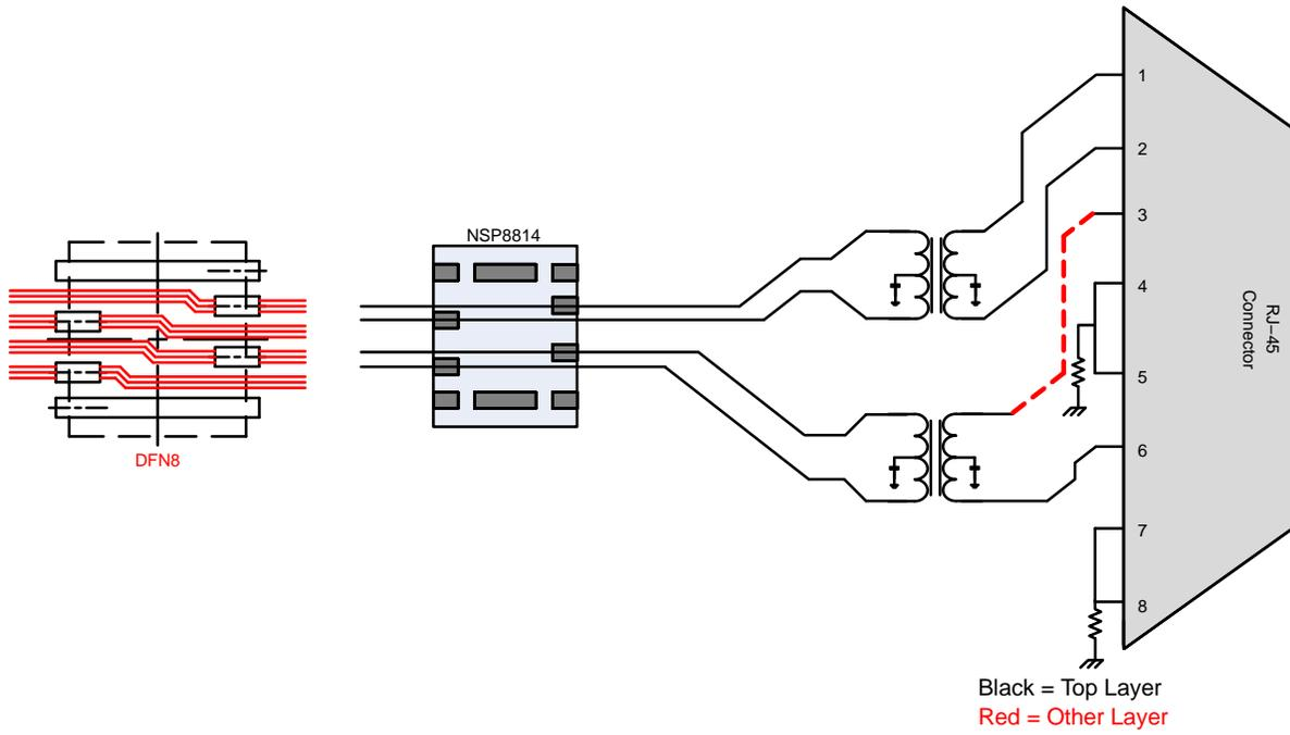
Figure 18. 10/100 Ethernet Layout Diagram and Flow-thru Routing Scheme
