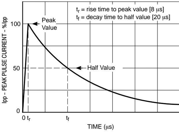
Figure 2. IEC61000-4-5 8/20  $\mu$ s Pulse Waveform
