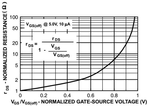
Figure 7. Normalized Drain Resistance vs. Bias Voltage
