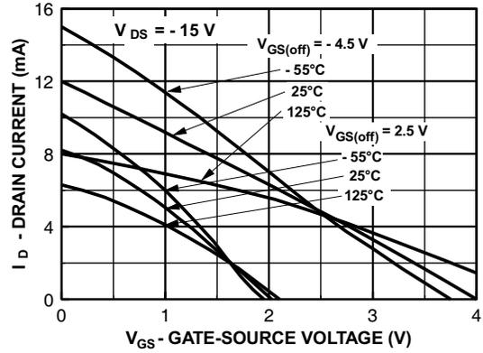
Figure 6. Transfer Characteristics
