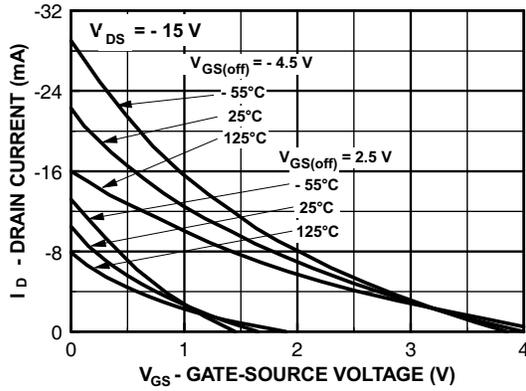
Figure 5. Transfer Characteristics
