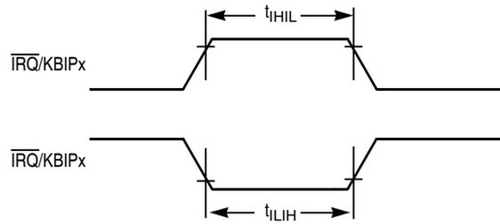
Figure 18.  $\overline{\text{IRQ}}/\text{KBIPx}$  Timing
