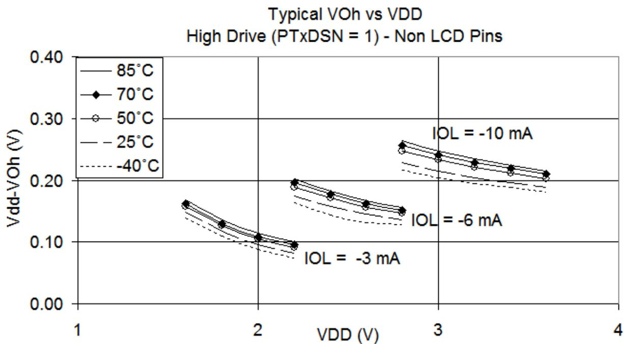
Figure 8. Typical High-Side (Source) Characteristics(Non LCD Pins) — High Drive (PTxDSn = 1)
