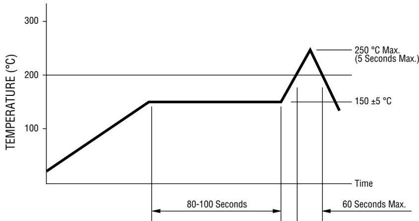
Processing Method: Reflow soldering with infrared heat or forced air convection (only once).
