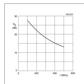
Class-B operation;  $\rm V_{DS}$  = 28 V;  $\rm I_{DQ}$  = 2  $\times$  80 mA;  $\rm P_{L}$  = 80 W.
