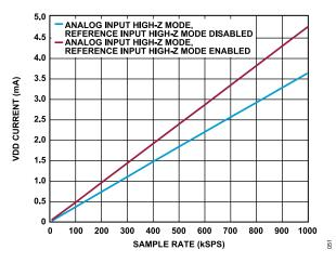
Figure 52. VDD Current vs. Sample Rate, Internal LDO Disabled
