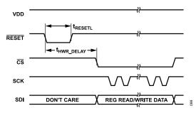
Figure 104. Hardware Reset Timing Diagram
