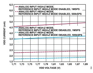
Figure 53. VDD Current vs. VDD Voltage, Internal LDO Disabled
