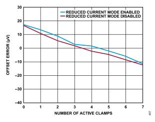
Figure 31. Offset Error vs. Number of Active Clamps, Clamp Current = 5 mA
