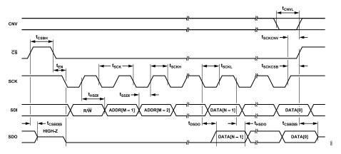
Figure 93. Register Configuration Mode Timing Diagram
