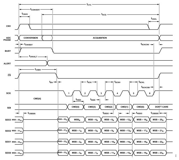
Figure 98. Conversion Mode Timing Diagram, Quad-SDO Mode, SDO STATE = 0
