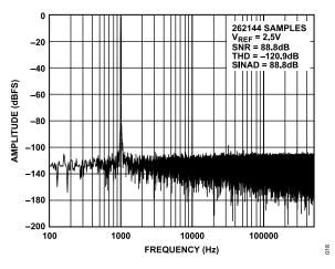
Figure 19. FFT,  $f_{IN}$  = 1 kHz,  $V_{REF}$  = 2.5 V, OSR = 1
