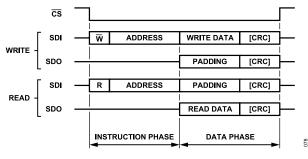
Figure 81. Basic SPI Frame
