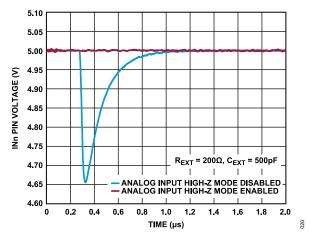
Figure 21. Analog Input Voltage Step with Analog Input High-Z Mode Disabled and Enabled
