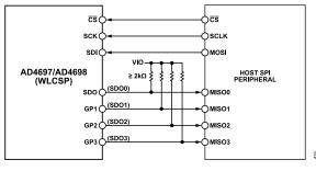
Figure 120. AD4697/AD4698 SPI Connection Diagram (Quad-SDO Mode)
