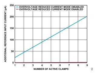
Figure 43. Additional Reference Input Current vs. Number of Active Clamps, Clamp Current = 5 mA, V<sub>REF</sub> = 5 V
