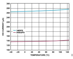
Figure 56. VIO Current vs. Temperature, Conversion Mode, OSR = 1
