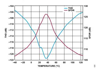
Figure 26. THD and SFDR vs. Temperature, f<sub>IN</sub> = 1 kHz
