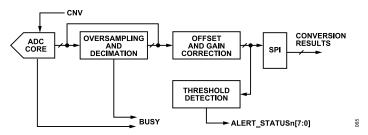
Figure 64. ADC Data Processing Path
