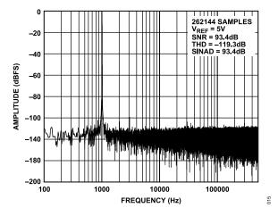
Figure 16. Fast Fourier Transform (FFT),  $f_{IN}$  = 1 kHz,  $V_{REF}$  = 5 V, OSR = 1
