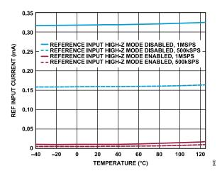
Figure 42. REF Input Current vs. Temperature, V<sub>REF</sub> = 5 V, Frequency of CNV Signal (f<sub>CNV</sub>) = 1 MSPS
