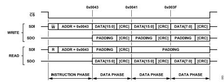
Figure 86. Streaming Mode SPI Frame, Looping Disabled, Descending Address, MB\_STRICT = 1
