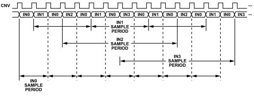
Figure 126. Multiple Effective Sample Rates Example
