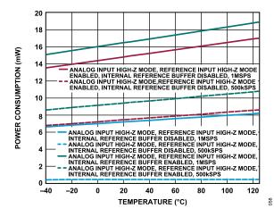
Figure 59. Power Consumption vs. Temperature, Internal LDO Disabled,  $f_{\rm S}$  = 1 MSPS and 500 kSPS
