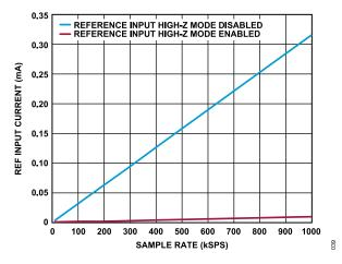
Figure 40. REF Input Current vs. Sample Rate, V<sub>REF</sub> = 5 V
