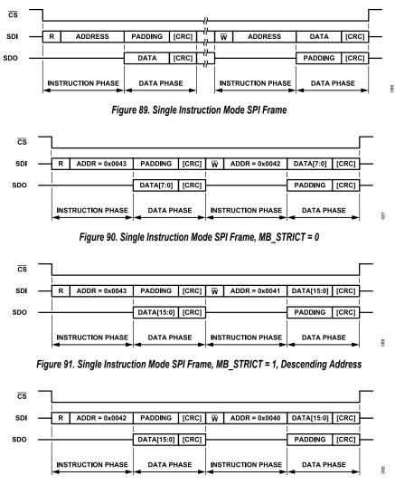
Figure 92. Single Instruction Mode SPI Frame, MB\_STRICT = 1, Ascending Address
