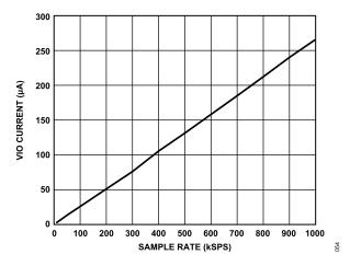
Figure 55. VIO Current vs. Sample Rate, Conversion Mode, OSR = 1
