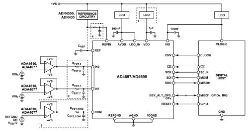
1. DEDICATED +1.8V SUPPLY FOR VDD NOT REQUIRED WHEN USING INTERNAL LDO 2. R<sub>EXTX</sub> AND C<sub>EXTX</sub> REPRESENT EXTERNAL INPUT RC FLITERS FOR ANALOG INPUT INx OR COM 3. DEDICATED ADC ORVERT FOR COM INPUT NOT REQUIRED IF CONNECTING COM TO REFGND 4. OPTIONAL RC FLITER BETWEEN VOLTAGE REFERENCE AND REFIN INPUT (REFERENCE BUFFER ENABLED ONLY)
