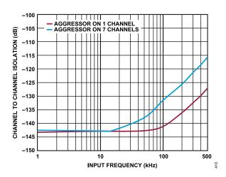
Figure 37. Channel to Channel Isolation vs. Input Frequency
