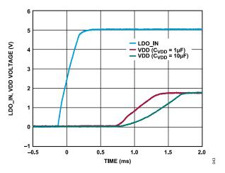
Figure 45. LDO\_IN, VDD Voltage vs. Time and VDD Decoupling Capacitance (C<sub>VDD</sub>)
