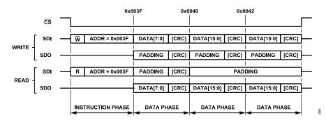
Figure 87. Streaming Mode SPI Frame, Looping Disabled, Ascending Address, MB\_STRICT = 1
