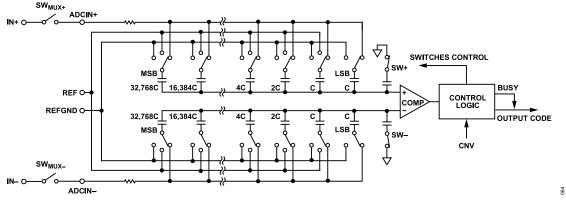
Figure 63. ADC Simplified Schematic
