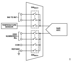
Figure 67. Multiplexer Simplified Schematic
