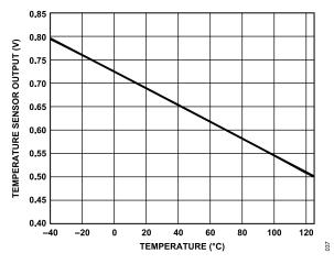
Figure 38. Temperature Sensor Output vs. Temperature
