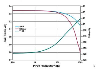
Figure 18. SNR, SINAD, and THD vs. Input Frequency
