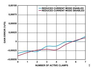
Figure 32. Gain Error vs. Number of Active Clamps, Clamp Current = 5 mA, Internal Reference Buffer Disabled
