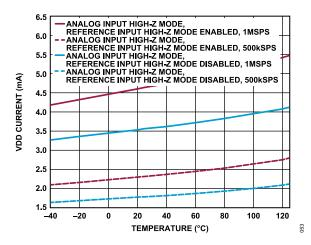
Figure 54. VDD Current vs. Temperature, Internal LDO Disabled
