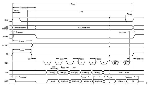
Figure 95. Conversion Mode Timing Diagram, Single-SDO Mode, SDO\_STATE = 1
