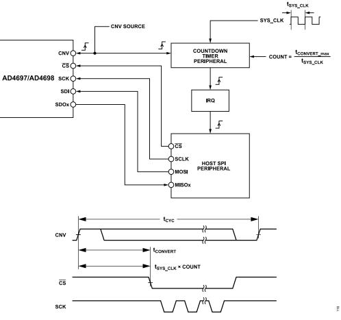
Figure 122. SPI Synchronization with Countdown Timer Peripheral
