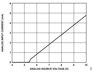
Figure 39. Analog Input Current vs. Analog Source Voltage,  $R_{EXT} = 1 k\Omega, V_{REF} = 5 V$
