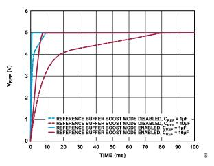
Figure 44. V<sub>REF</sub> vs. Time for Various Reference Buffer Boost Mode Settings and C<sub>REF</sub>
