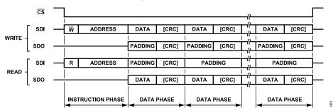
Figure 84. Streaming Mode SPI Frame
