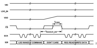
Figure 110. LDO Wake-Up Command POR Timing Diagram
