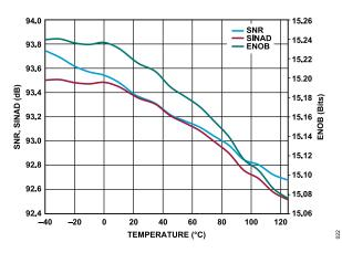
Figure 23. SNR, SINAD, and ENOB vs. Temperature, f<sub>IN</sub> = 1 kHz
