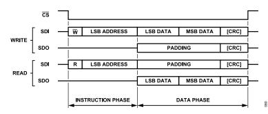
Figure 83. Multibyte Register Access with MB\_STRICT = 1 and Ascending Address
