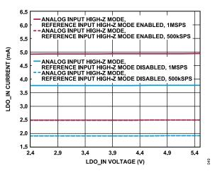
Figure 50. LDO\_IN Current vs. LDO\_IN Voltage, Internal LDO Enabled
