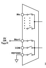
Figure 70. Even-Channel and Odd-Channel Paired
