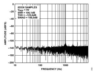
Figure 20. FFT, f<sub>IN</sub> = 1 kHz, V<sub>REF</sub> = 2.5 V, OSR = 64
