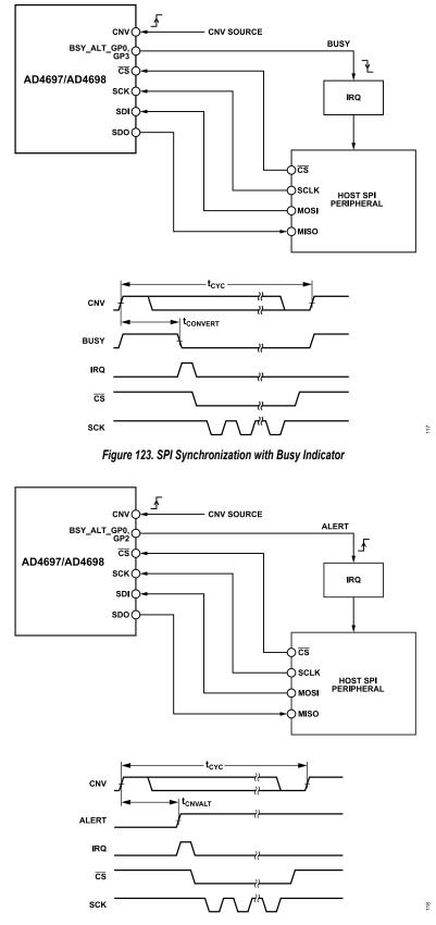
Figure 124. SPI Synchronization with Alert Indicator
