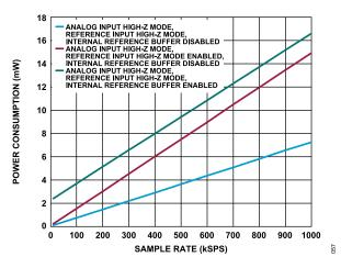
Figure 58. Power Consumption vs. Sample Rate, Internal LDO Disabled
