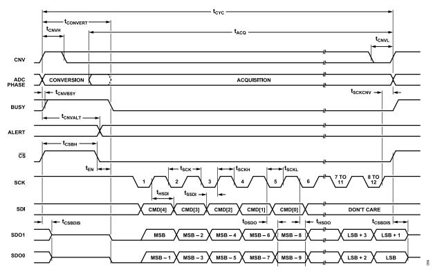
Figure 97. Conversion Mode Timing Diagram, Dual-SDO Mode, SDO\_STATE = 1
