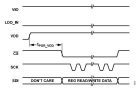
Figure 106. VDD POR Timing Diagram
