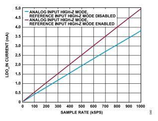
Figure 49. LDO\_IN Current vs. Sample Rate, Internal LDO Enabled
