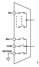
Figure 68. INx Paired with REFGND
