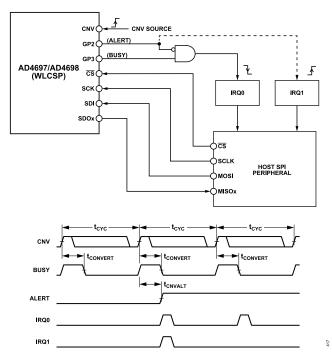
Figure 125. SPI Synchronization with Busy and Alert Indicators
