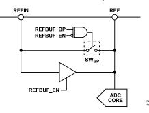
Figure 74. Internal Reference Buffer Simplified Schematic
