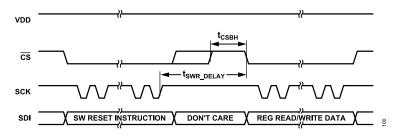
Figure 105. Software Reset Timing Diagram
