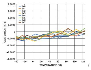
Figure 29. Gain Error vs. Temperature, Internal Reference Buffer Disabled
