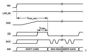
Figure 109. VIO POR Timing Diagram (Internal LDO Supplying VDD)
