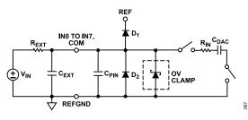
Figure 66. Equivalent Analog Input Circuit
