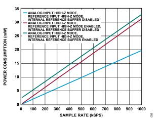
Figure 61. Power Consumption vs. Sample Rate, Internal LDO Enabled
