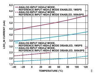
Figure 51. LDO\_IN Current vs. Temperature, Internal LDO Enabled
