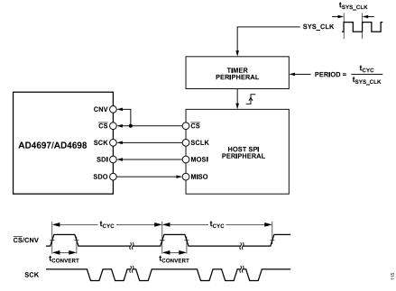
Figure 121. 4-Wire SPI Operation Diagram
