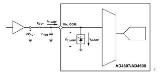
Figure 115. Analog Input Overvoltage Event
