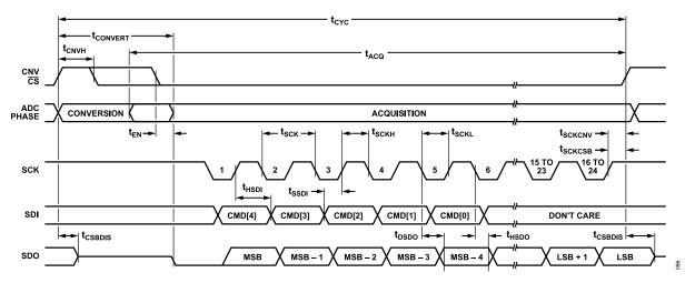
Figure 101. Conversion Mode Timing Diagram with 4-Wire SPI, Single-SDO Mode, SDO STATE = 1
