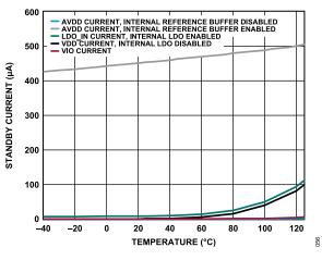
Figure 57. Standby Current vs. Temperature
