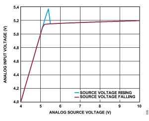
Figure 36. Analog Input Voltage vs. Analog Source Voltage,  $R_{EXT} = 1 \ k\Omega, V_{REF} = 5 \ V$
