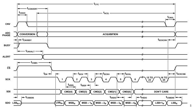
Figure 94. Conversion Mode Timing Diagram, Single-SDO Mode, SDO\_STATE = 0
