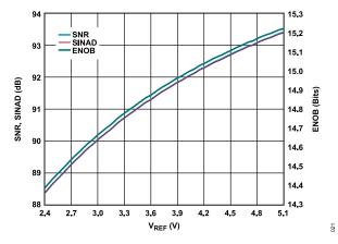
Figure 22. SNR, SINAD, and Effective Number of Bits (ENOB) vs. V<sub>REF</sub>, f<sub>IN</sub> = 1 kHz
