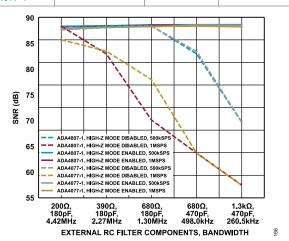
Figure 71. SNR vs. External RC Filter Components, Bandwidth for Various Amplifiers ( $V_{REF} = 5 V$ ,  $f_{IN} = 1 kHz$ )
