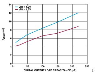
Figure 60. t<sub>DSDO</sub> vs. Digital Output Load Capacitance
