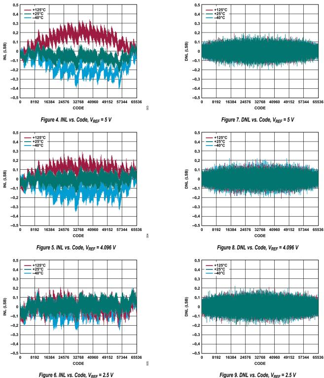
Figure 9. DNL vs. Code, V<sub>REF</sub> = 2.5 V
