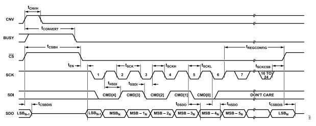
Figure 102. Conversion Mode Timing Diagram, Register Configuration Mode Command
