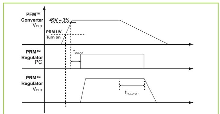
Figure 31 – PRM Enable Hold off Waveforms
