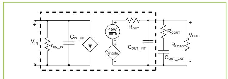
**Figure 28** – PF175B480C033FP-00 AC small signal model
