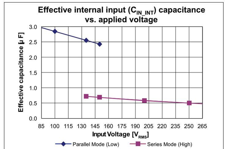
Figure 23 – Effective input capacitance vs.  $V_{IN}$ .
