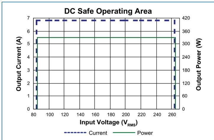
Figure 1 — DC output safe operating area
