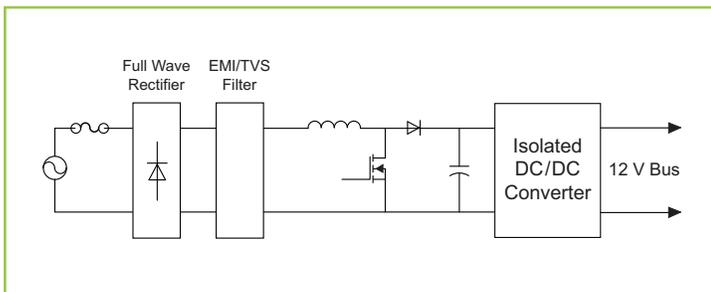
**Figure 27** – Traditional PFC AC to DC supply
