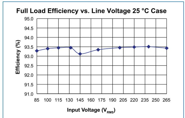
Figure 2 — Full load efficiency vs. line voltage
