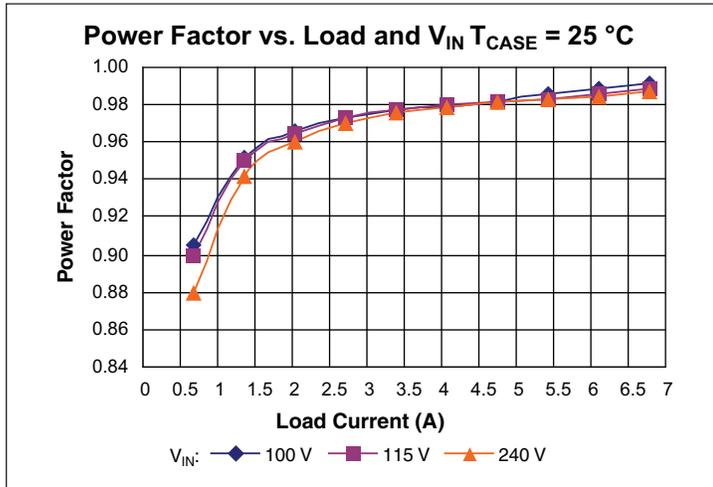
Figure 18 – Typical power factor vs.  $V_{IN}$  and  $I_{OUT}$ .
