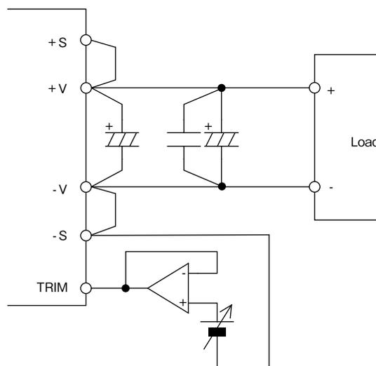
Fig. 2-2 Output Voltage Adjustment by applying external voltage
