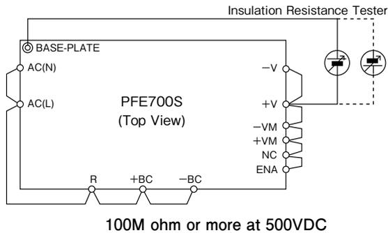
Fig. 17-1 Insulation Resistance Test Method
