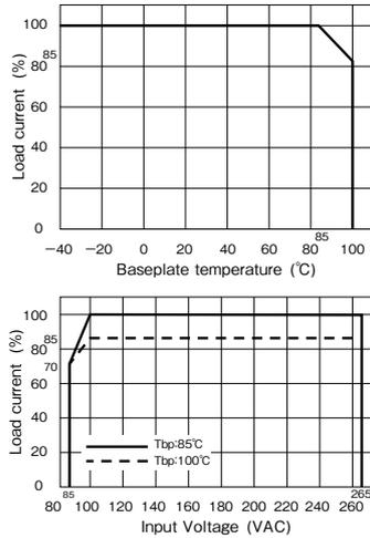
Fig. 11-2 Derating Curve
