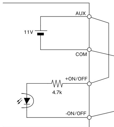
Fig. 10-3 ON/OFF Control Connection Example 3
