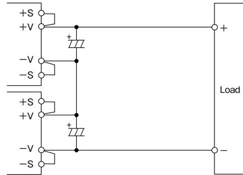
Fig. 10-1 Series Operation for High Output Voltage Applications
