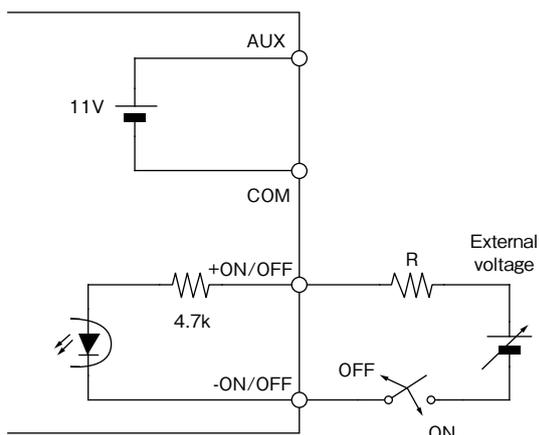
Fig. 10-1 ON/OFF Control Connection Example 1
