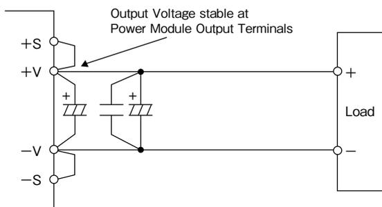
Fig. 9-2 Remote Sensing is not used (Local Sensing)
