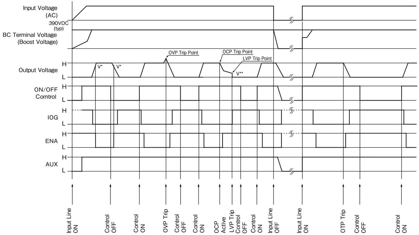
$V^*$  voltage level: Refer to Application Notes "13.Power ON Signal" section.
