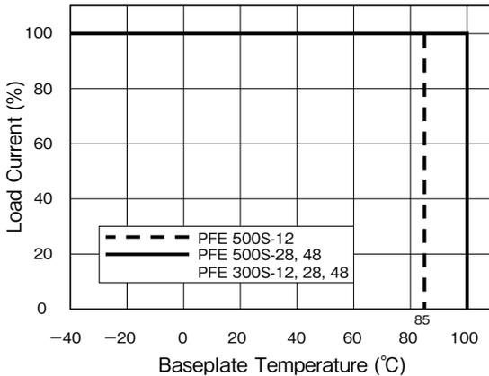
Fig. 12-2 Derating Curve
