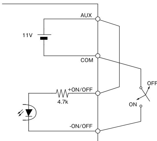
Fig. 10-2 ON/OFF Control Connection Example 2
