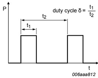
Fig. 17. Duty cycle definition
