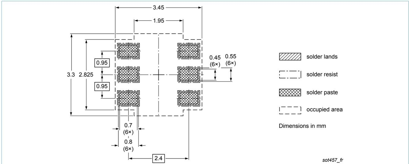
Fig. 19. Reflow soldering footprint for TSOP6 (SOT457)
