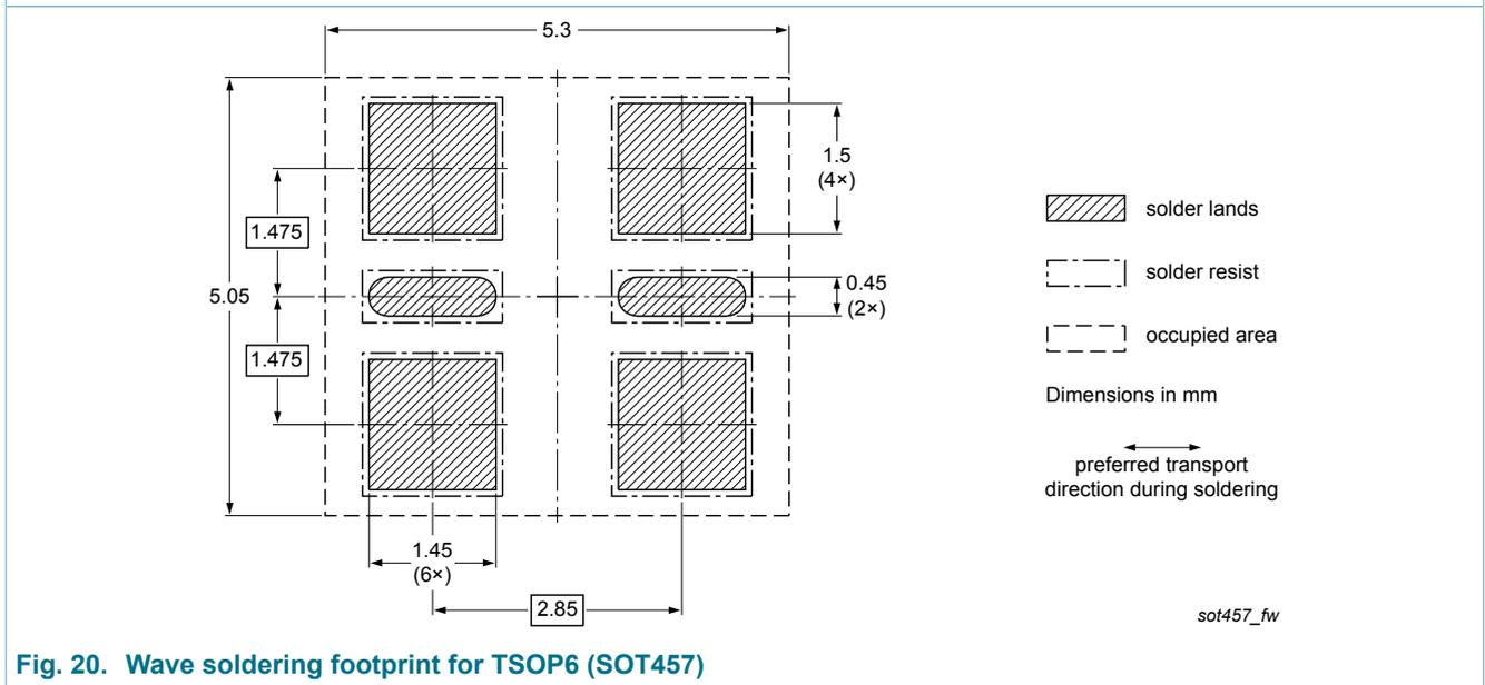
Fig. 20. Wave soldering footprint for TSOP6 (SOT457)
