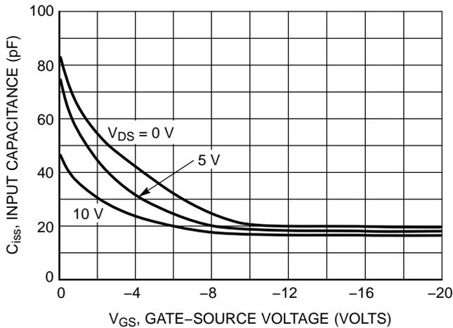
**Figure 1. Common Source Input Capacitance versus Gate-Source Voltage**
