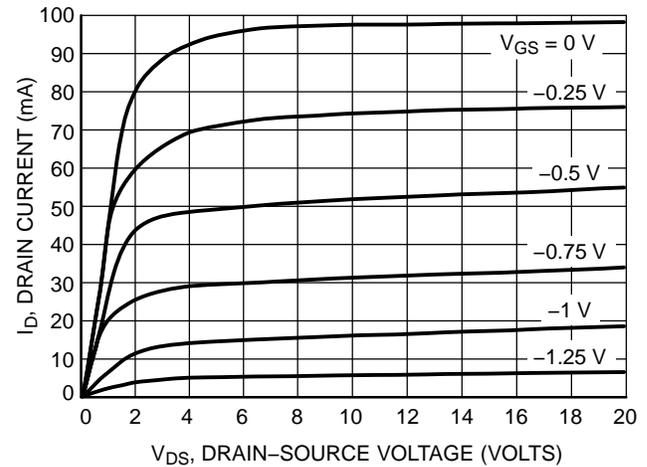
**Figure 4. Output Characteristic  $V_{GS(off)} = -2.0 \text{ V}$**
