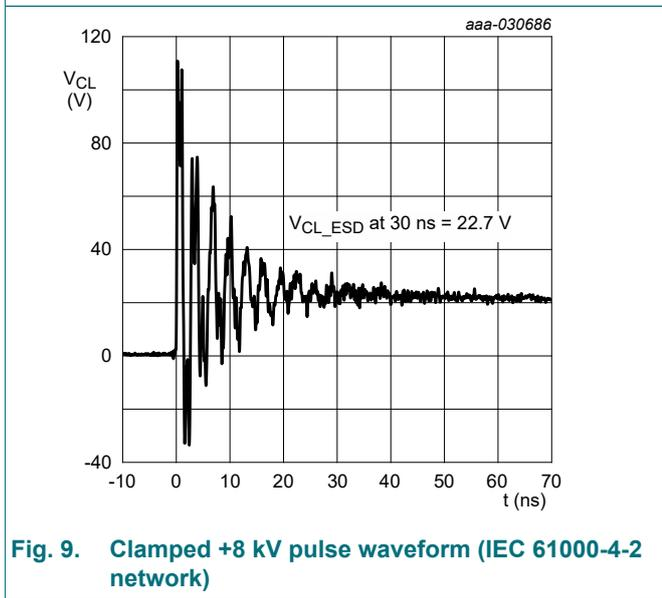
Fig. 9. Clamped +8 kV pulse waveform (IEC 61000-4-2 network)
