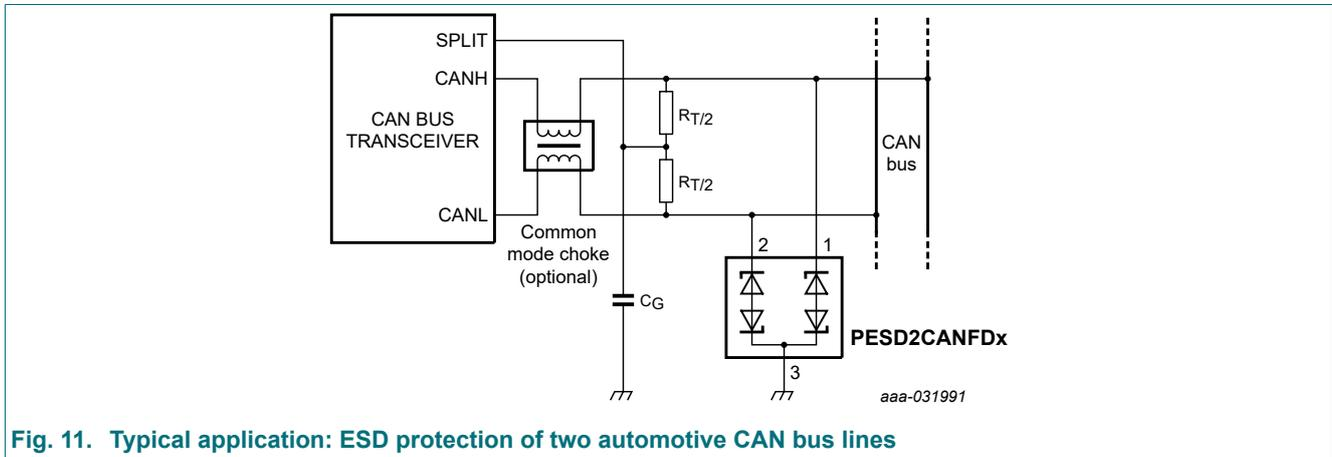
Fig. 11. Typical application: ESD protection of two automotive CAN bus lines
