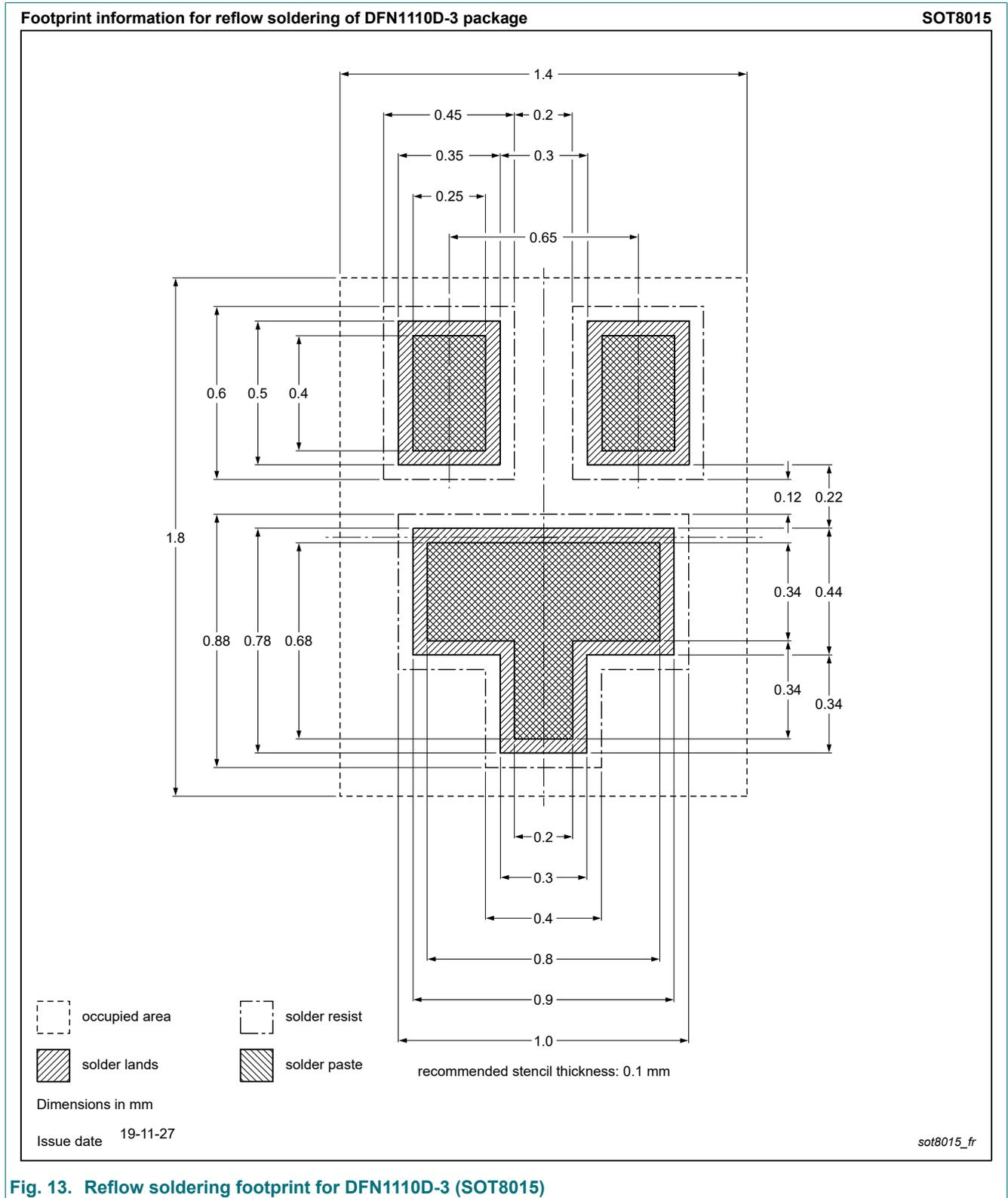
**Fig. 13. Reflow soldering footprint for DFN1110D-3 (SOT8015)**
