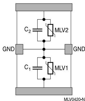
Model of EMI filtering with matched capacitances  $C_1$  and  $C_2$
