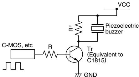
\* Resistor to do charging and discharging to a piezoelectric element
