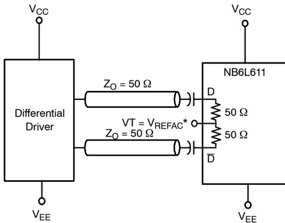
Figure 18. Capacitor-Coupled Differential Interface
