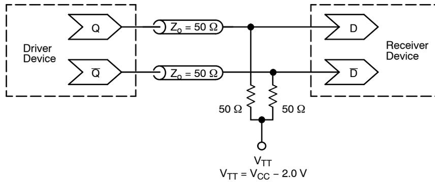
**Figure 20. Typical Termination for Output Driver and Device Evaluation
