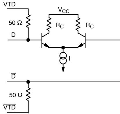
Figure 8. Input Structure
