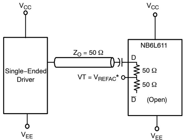
Figure 19. Capacitor-Coupled Single-Ended Interface
