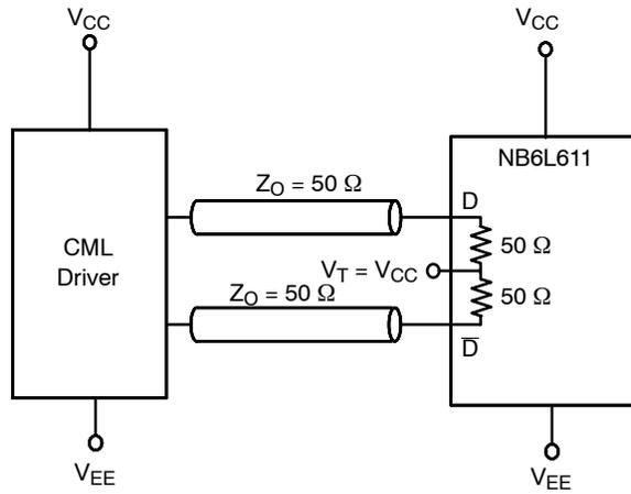
Figure 17. Standard 50  $\Omega$  Load CML Interface
