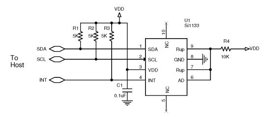
Figure 2.1. Basic Application Circuit
