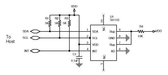
Figure 2.2. Basic Application Circuit Using the Alternate I<sup>2</sup>C Address
