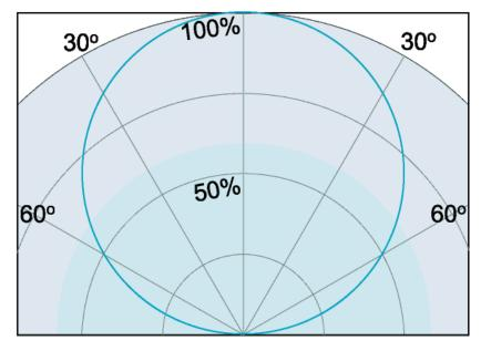
Figure 1.2. Desired Cosine Response of the UV Index Sensor
