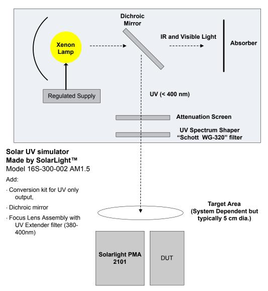
Figure 9.2. Using a Solar Simulator to Calibrate the Sensor
