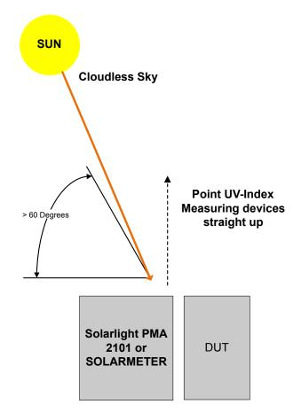
Figure 9.1. Using the Sun to Calibrate the Sensor
