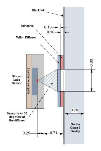
Figure 5.1. Compact Sensor Assembly
