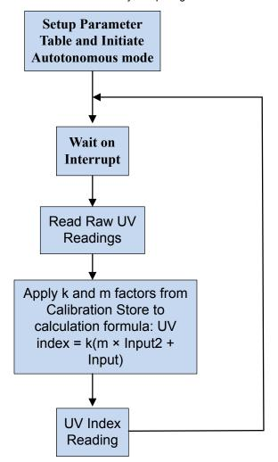
Figure 9.3. Calibration Flowchart
