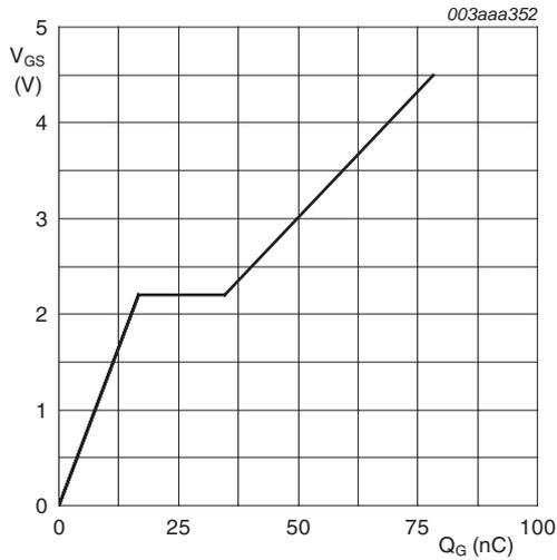
$I_D = 50A; V_{DS} = 10V$
