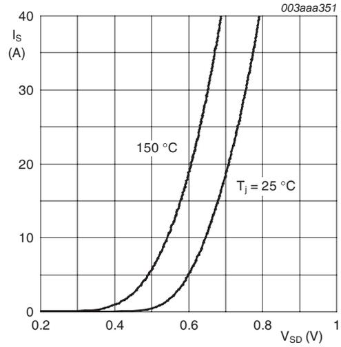
$T_j = 25^\circ C \text{ and } 150^\circ C; V_{GS} = 0V$
