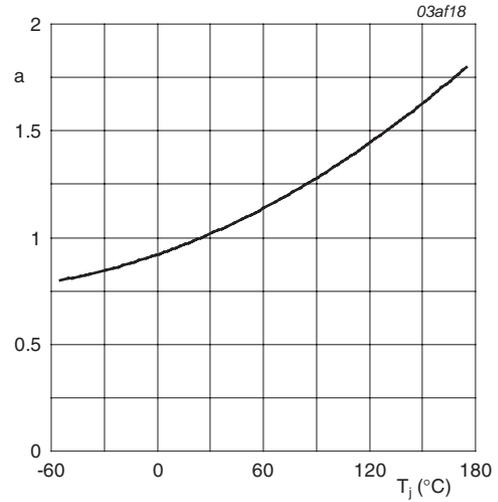
$$a = \frac{R_{DS(on)}}{R_{DS(on)(25^\circ C)}}$$
