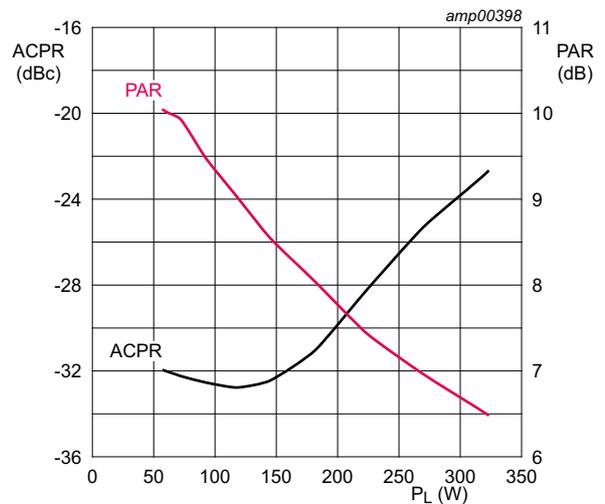
$V_{DS} = 50$  V;  $I_{Dq} = 2 \times 900$  mA; PAR (of output signal) at 0.01 % probability on CDDF; PAR of input signal = 9.5 dB at 0.01 % probability on CDDF.
