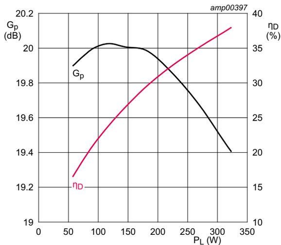
$V_{DS} = 50$  V;  $I_{Dq} = 2 \times 900$  mA; PAR (of output signal) at 0.01 % probability on CDDF; PAR of input signal = 9.5 dB at 0.01 % probability on CDDF.
