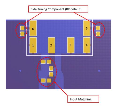
In addition to the matching circuit, a separate DC blocking capacitor will also be required between the radio and the antenna matching circuit.
