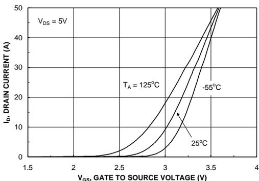
Figure 5. Transfer Characteristics.
