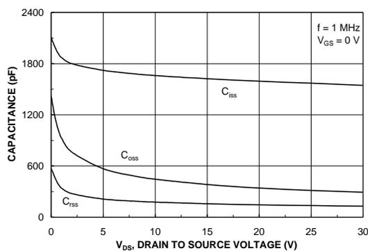
Figure 8. Capacitance Characteristics.
