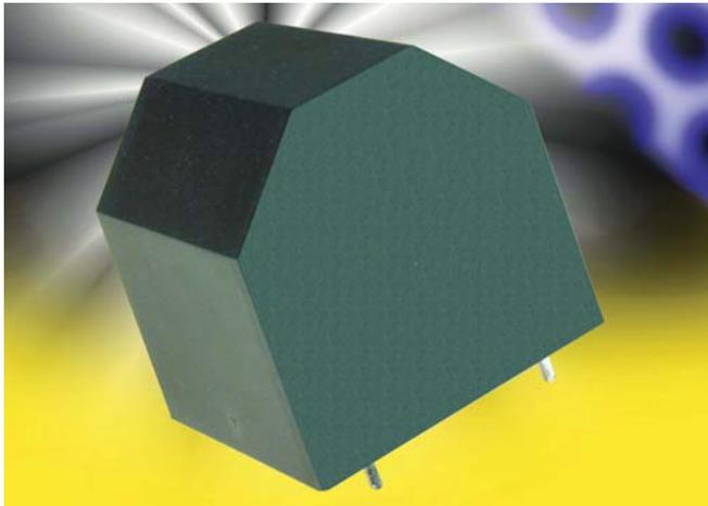
The series uses a metallized polypropylene or polyester dielectric, with the controlled self-healing process, specially treated to have a very high dielectric strength in operating conditions up to 105°C. This is a dry solution for polypropylene and dry or wet for polyester. The FFV3 has been designed for printed circuit board mounting.
