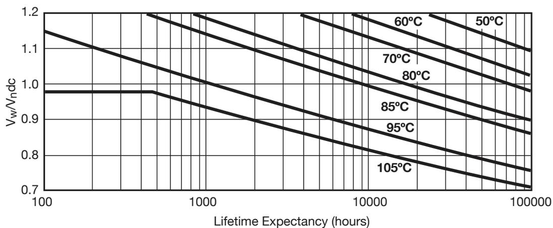
V<sub>w</sub> = Permanent working or operating DC voltage.
