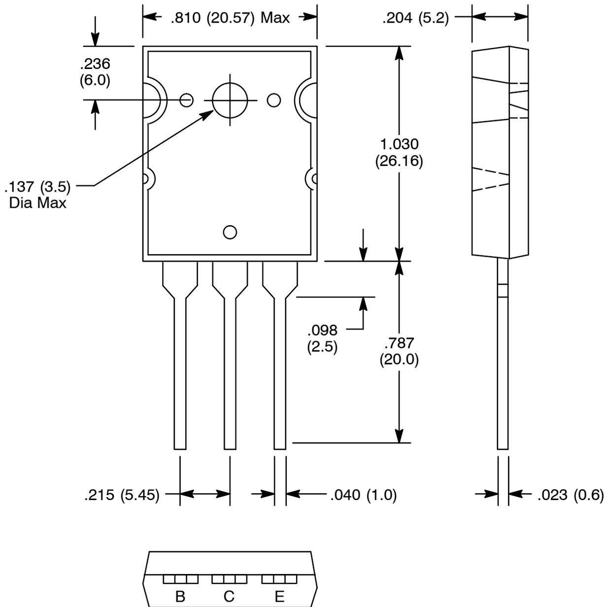
**NOTE:** Pin2 connected to heatsink
