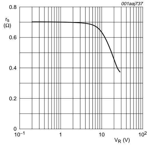
$f = 470 \text{ MHz}; T_j = 25 \text{ }^\circ\text{C}.$
