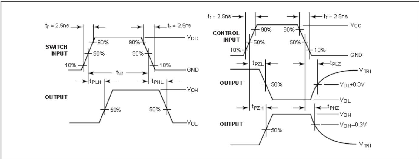
**Figure 2. AC Waveforms**
