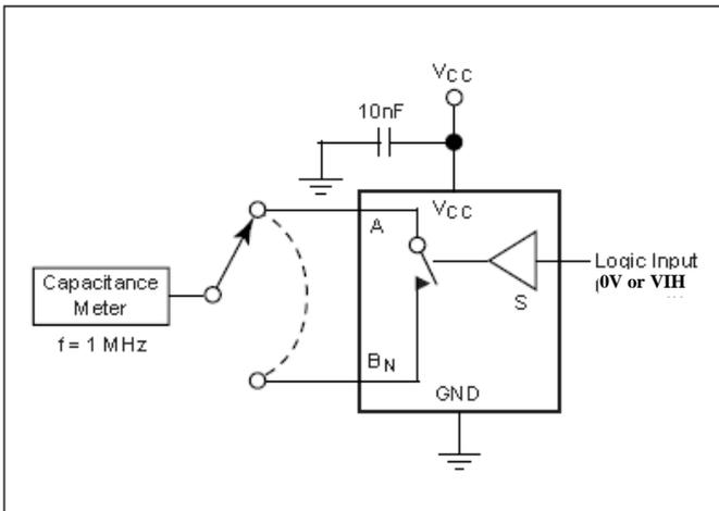
**Figure 7. Channel Off Capacitance**
