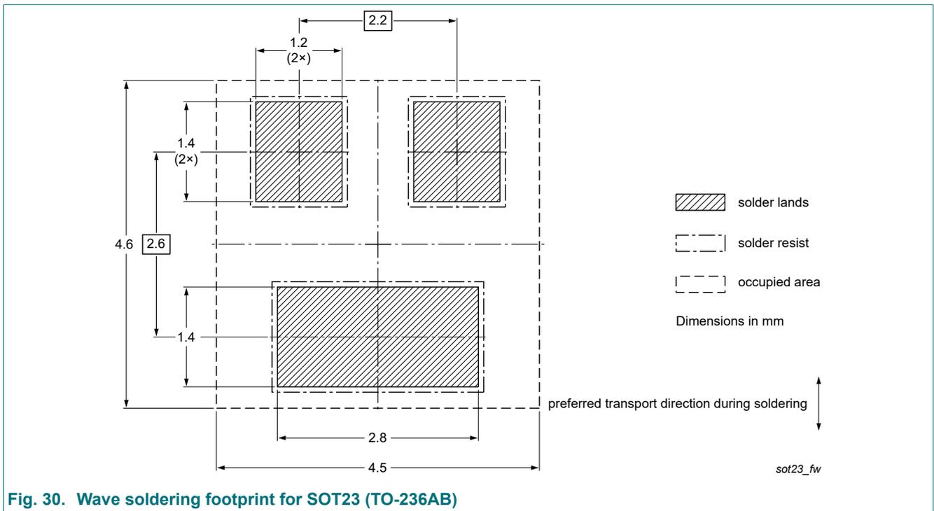
Fig. 30. Wave soldering footprint for SOT23 (TO-236AB)
