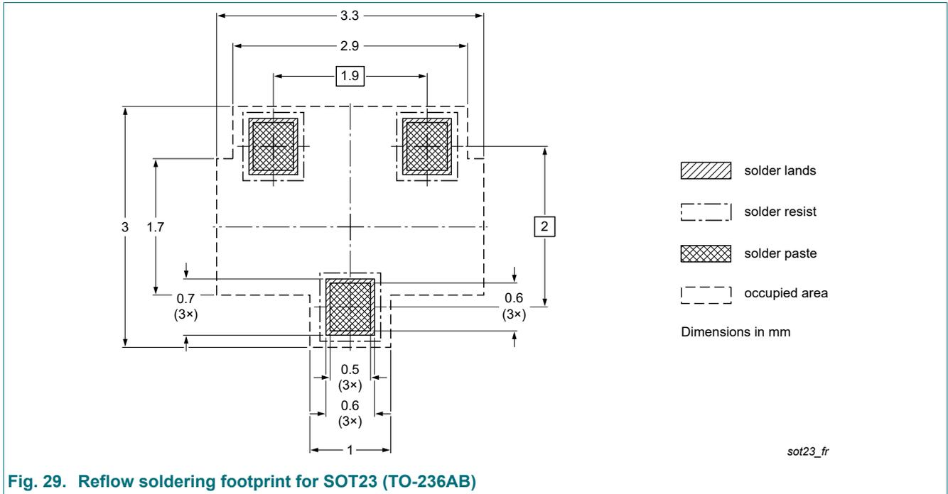
Fig. 29. Reflow soldering footprint for SOT23 (TO-236AB)
