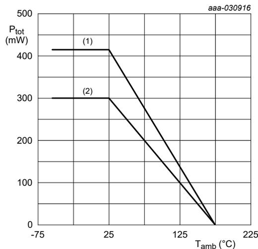
(1) FR4 PCB;  $1\text{ cm}^2$  mounting pad for collector
