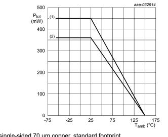
(1) FR4 PCB; single-sided 70 µm copper, standard footprint (2) FR4 PCB; single-sided 35 µm copper, standard footprint
