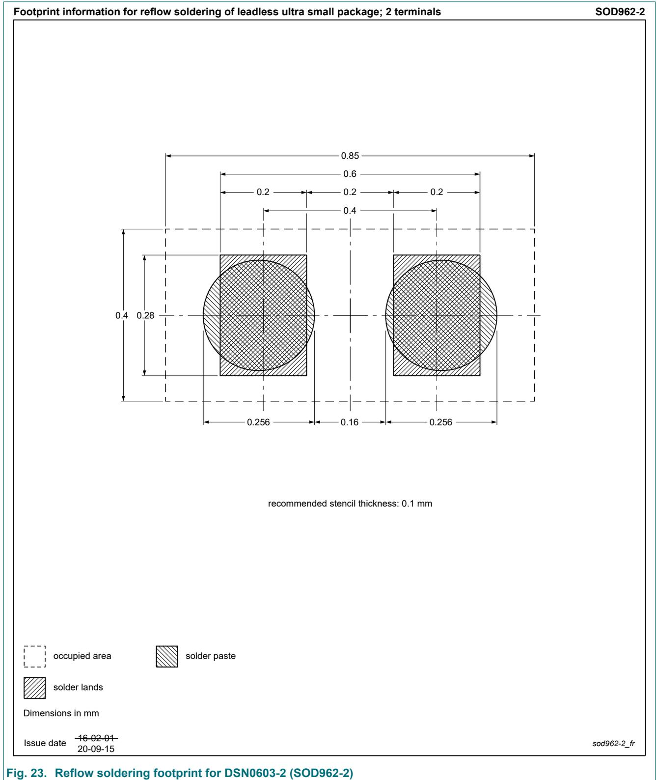
Fig. 23. Reflow soldering footprint for DSN0603-2 (SOD962-2)
