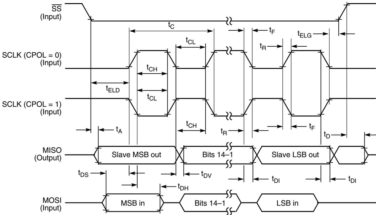
Figure 18. SPI slave timing (CPHA = 0)
