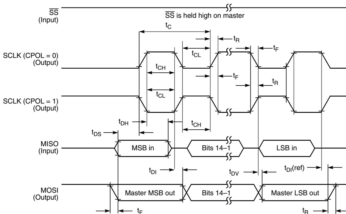
**Figure 16. SPI master timing (CPHA = 0)**
