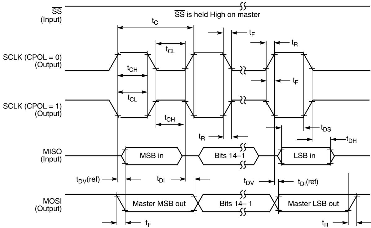
Figure 17. SPI master timing (CPHA = 1)
