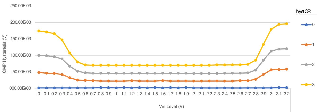
**Figure 12. Typical hysteresis vs.  $V_{in}$  level ( $V_{DD} = 3.3 \text{ V}$ ,  $\text{PMODE} = 0$ )**
