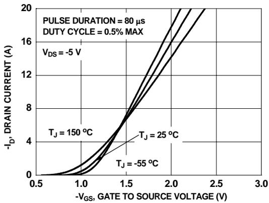
**Figure 5. Transfer Characteristics**
