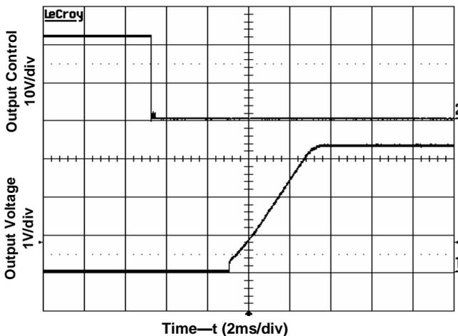
Figure 6. Start-Up from Enable Control
