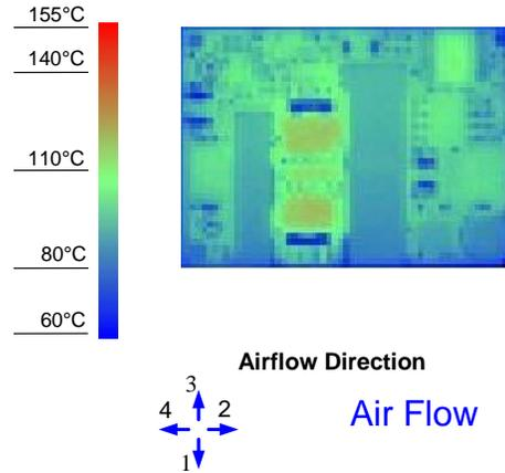
**Figure 10. Thermal Image for Airflow Direction 3**
