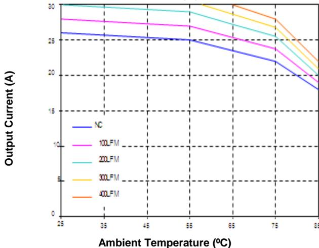
**Figure 9. Current Derating Curve with Open Frame**
