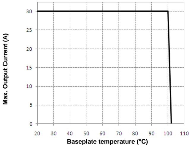
**Figure 11. Current Derating Curve for Baseplate**
